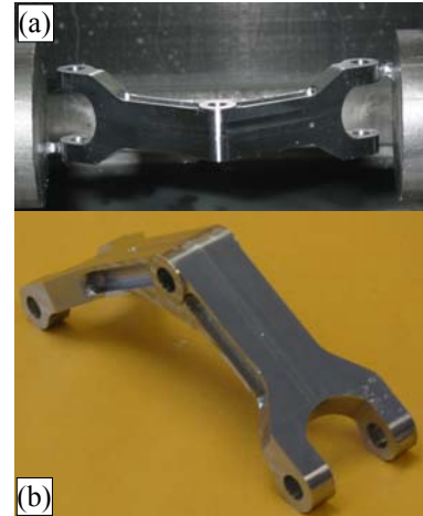
Figure 2 – A sample part: a) in process using sacrificial supports and b) upon removal
