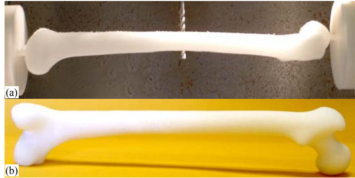
Figure 14 –Femur: (a) Fixtured with supports (b) Finished part
