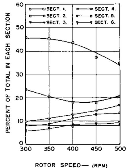
FIG. 4 Weight of grain in each sampler box section as a percentage of the total weight of grain in the sampler box.
