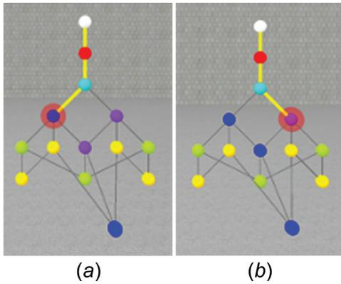
**Fig. 4 Graph visualization changes dynamically with user interaction. The top white node represents the starting, fully assembled state and the bottom nodes represent possible end states. (a) red, teal, and blue pieces removed and (b) red, teal, and purple pieces removed**
