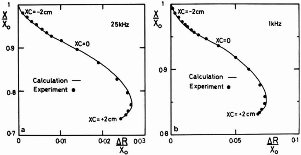
Fig. 2. Edge-effect loci in the normalized impedance plane for frequencies of (a) 25kHz and (b) 1 kHz. The solid circles are the experimental results and the curves are the results of the numerical calculation. The coil reactance ( $X$ ) and change in coil resistance ( $\Delta R$ ) are normalized to the isolated coil reactance ( $X_0 = \omega L_0$ ) following the usual convention.
