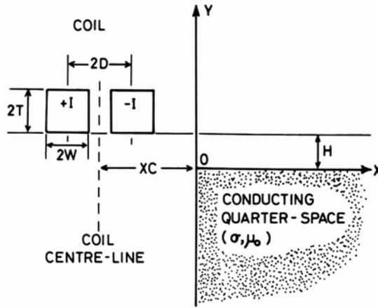
Fig. 1. Two-dimensional coil conducting quarter-space. Here XC is defined as positive when the coil is over the conductor.
