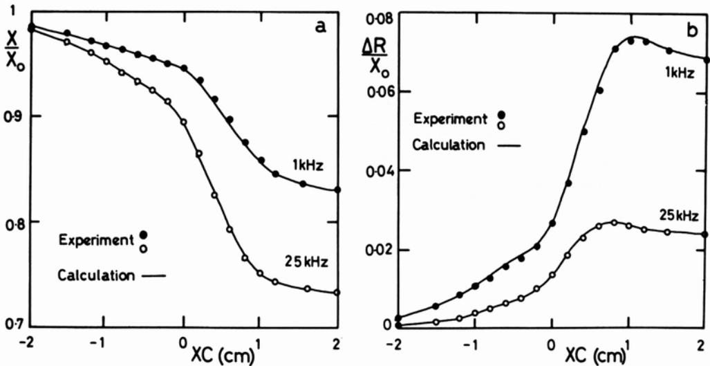
Fig. 3. Normalized coil reactance (a) and resistance (b) as a function of coil translation ( $XC$ ) near a  $90^\circ$  edge for frequencies of 25kHz and 1kHz. The circles are the experimental data and the solid lines are the results of the numerical calculation.
