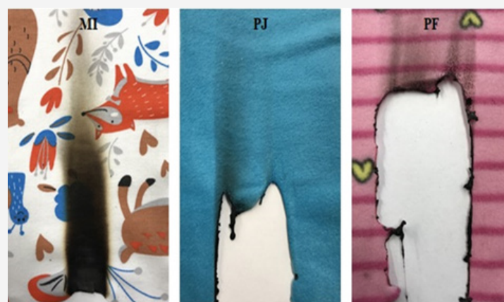
Figure 2: Fabric response to vertical flammability test (before wash).
