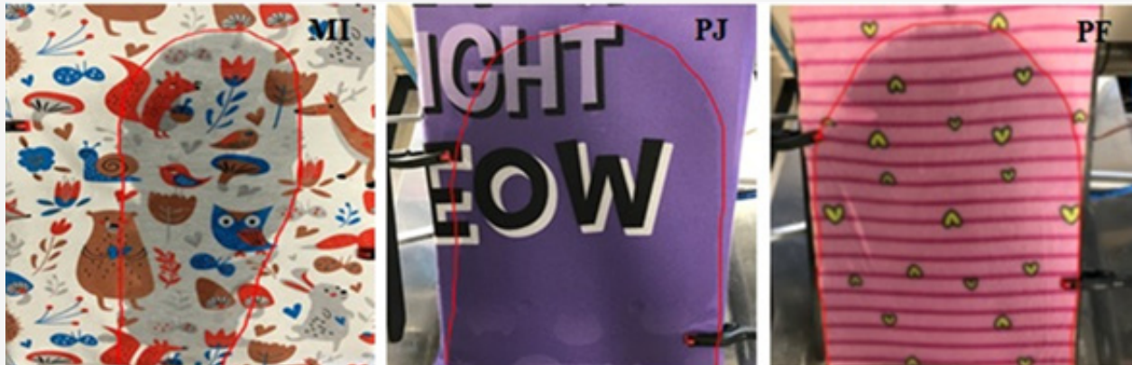
Figure 5: Surface wetting of the fabrics after hot splash.
