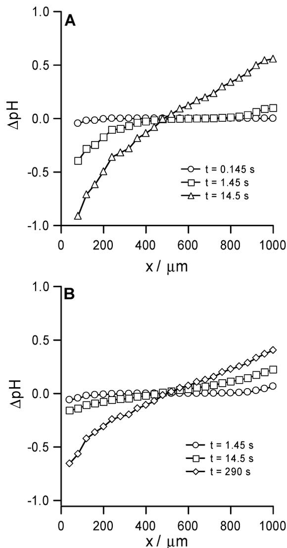
**Figure 6.** Simulated changes in pH within a microchannel cell for (A) potential gradient and (B) two-terminal electrode configuration at various times. The change in pH is with respect to an arbitrary initial value. Details of the simulation are provided in the text.
