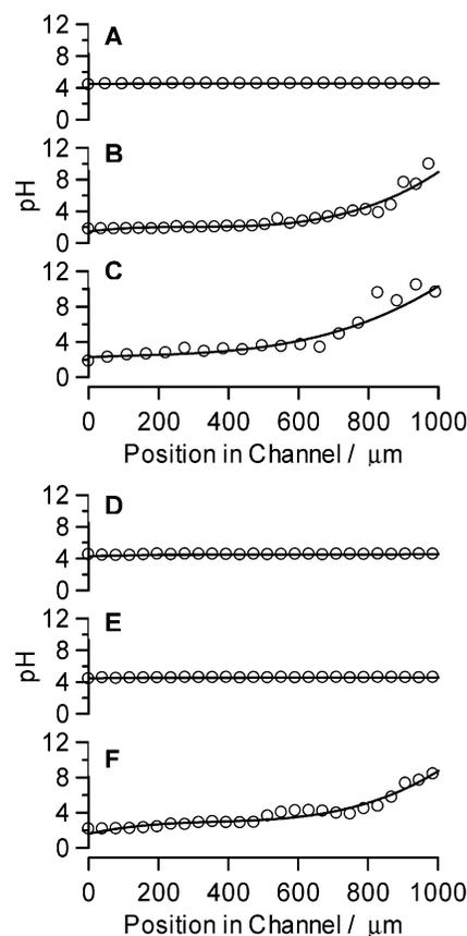
**Figure 5.** pH profiles within microchannel as measured with universal indicator for (A–C) potential gradient and (D–F) two-terminal electrode configuration. The data reflects pH profiles at 0 (A, C) and 15 s (B, E) and 5 min (C, F) after a potential difference of  $\Delta E = 1.12$  V is applied to the edges of each sample. The solid lines represent a polynomial fit of the data to guide the eye.
