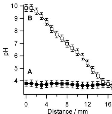
**Figure 2.** Measured pH profile along electrode surface determined using IrO<sub>2</sub> micro pH electrode. Curve A: no applied potential. Curve B: applied potential of  $-1 \text{ V}$  at left and  $1 \text{ V}$  at right.
