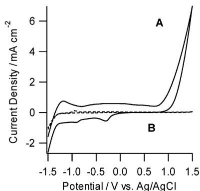
**Figure 1.** Cyclic voltammetry of (A) electrodeposited platinum and (B) ITO. Scan rate 0.1 V/s in 0.1 M Na<sub>2</sub>SO<sub>4</sub> at pH 4.
