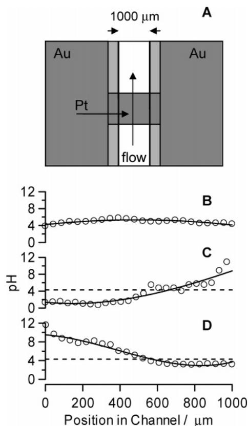
**Figure 4.** (A) Schematic of microscale flow cell containing gold contact pads, platinum catalyst region, and flow channel. (B–D) pH profile measured with universal indicator across the microchannel under various applied potentials. (B) No applied potential ( $\Delta E = 0$  V). (C)  $\Delta E = 1.86$  V. (D)  $\Delta E = -2.35$  V. The dashed line in (C) and (D) represents the initial pH within the channel, and the solid lines represent a polynomial fit of the data to guide the eye.
