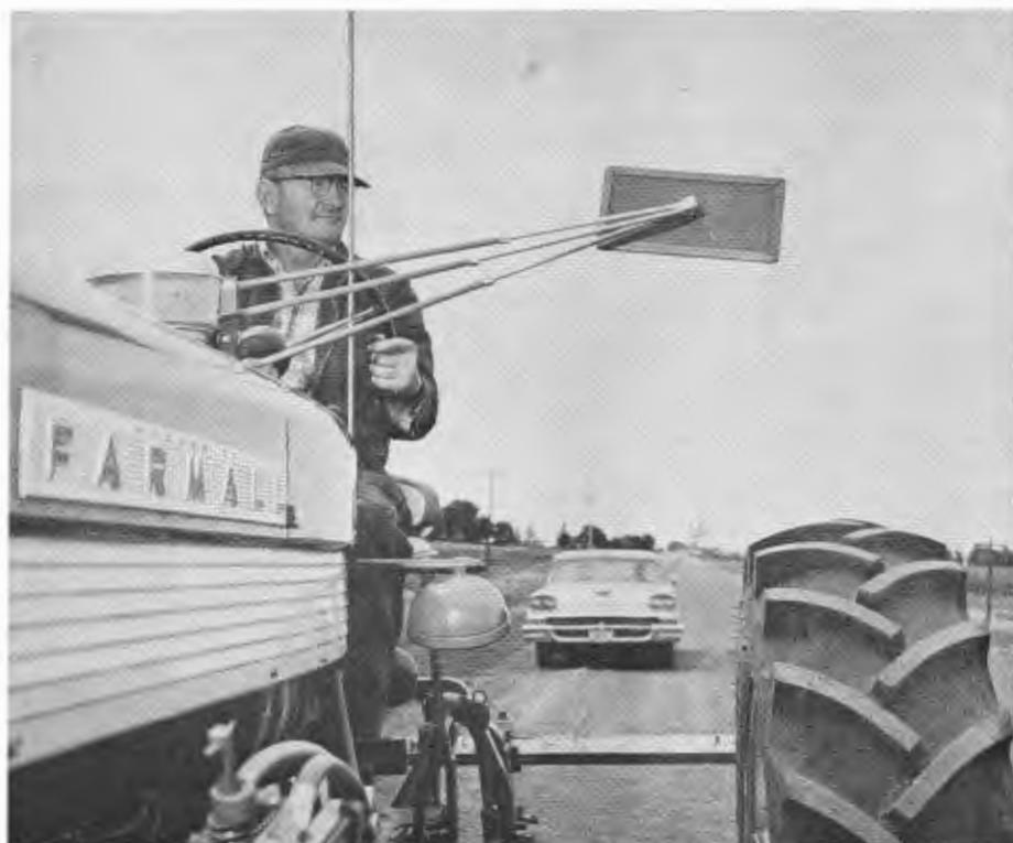
A rear-view mirror is an important safety device for on-the-road travel. With a mirror, you can determine the traffic situation behind you at a glance — avoiding the erratic steering resulting from the necessity of constantly having to turn around and look.
