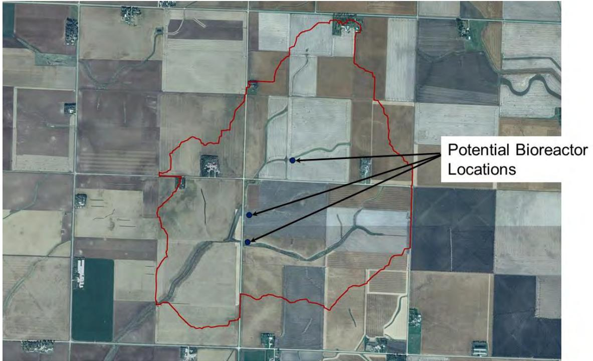
**Figure 2.** Potential locations for subsurface drainage bioreactors
