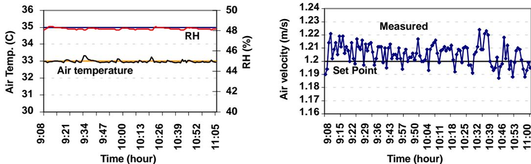
Figure 5. Examples of controlled air temperature, RH and air velocity profiles with regards to set points (unit conversion:  $^{\circ}\text{F} = 1.8 \times ^{\circ}\text{C} + 32$ ).
