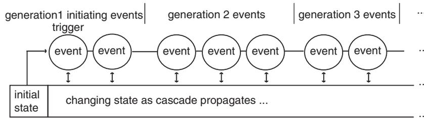
**Fig. 1.** Overall structure of cascading failure in which events are grouped into successive generations. A trigger event followed by immediate protection actions forms an initiating generation of events. Subsequent generations of cascading events can follow, and the system state changes and weakens as the cascading events propagate.
