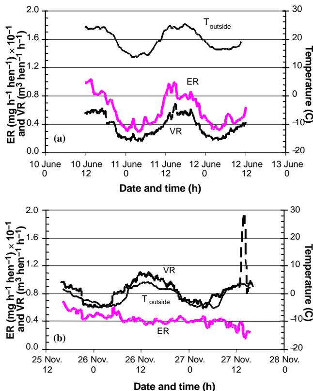
Figure 12. Ammonia emission rate (ER) and building ventilation rate (VR) of high-rise layer houses in IA during (a) mild (June) days and (b) cold (November) days.
