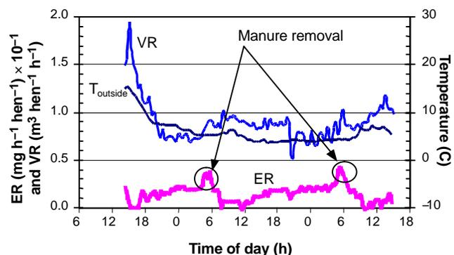
Figure 13. Example diurnal profiles of ammonia emission rate (ER) and building ventilation rate (VR) of a manure-belt layer house in IA.
