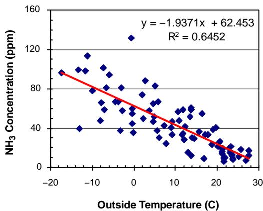
Figure 8. Daily mean ammonia concentration of the exhaust air in an IA high-rise house (with standard diet) vs. outside temperature (standard errors for slope and intercept are 0.16 and 2.4, respectively).
