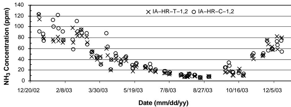
Figure 7a. Daily mean ammonia concentrations in exhaust air from high-rise (HR) layer houses in IA with either standard diet, C (O), or lower CP diet, T (X).
