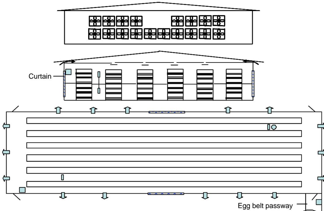
Figure 2. Schematic layout of the PA manure-belt layer house showing the end wall, cross-section, and floor plan of the house and the sampling locations (symbols are the same as in fig. 1).
