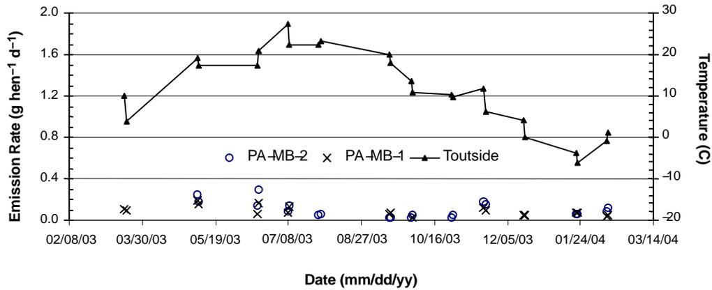
Figure 9b. Daily mean ammonia emission from manure-belt layer houses in PA, where manure was removed from the houses semi-weekly, and outside temperatures.
