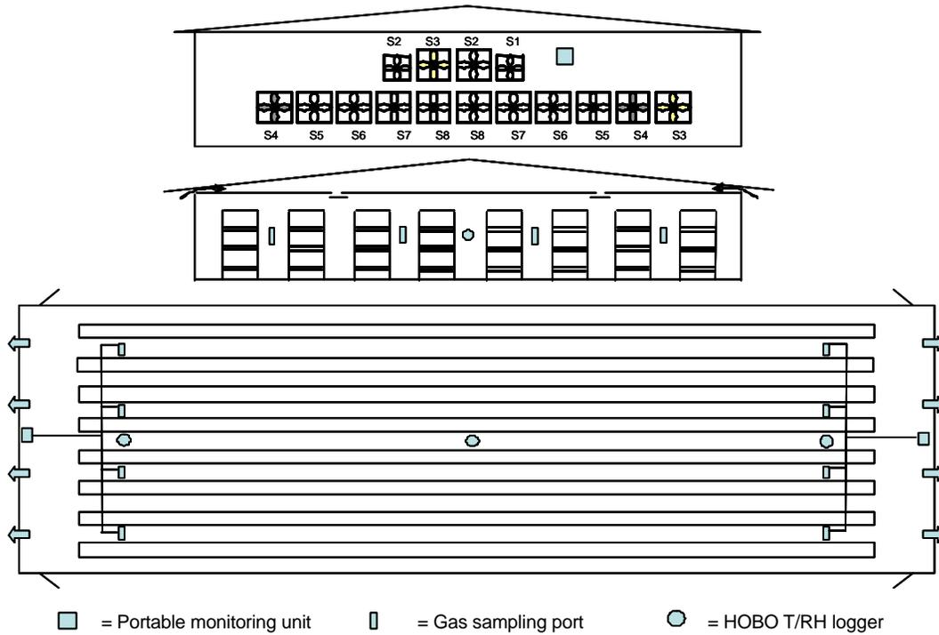
Figure 1. Schematic layout of the IA manure-belt layer house showing the end wall, cross-section, and floor plan of the house and the sampling locations. The exhaust fans are labeled by stages 1-8.
