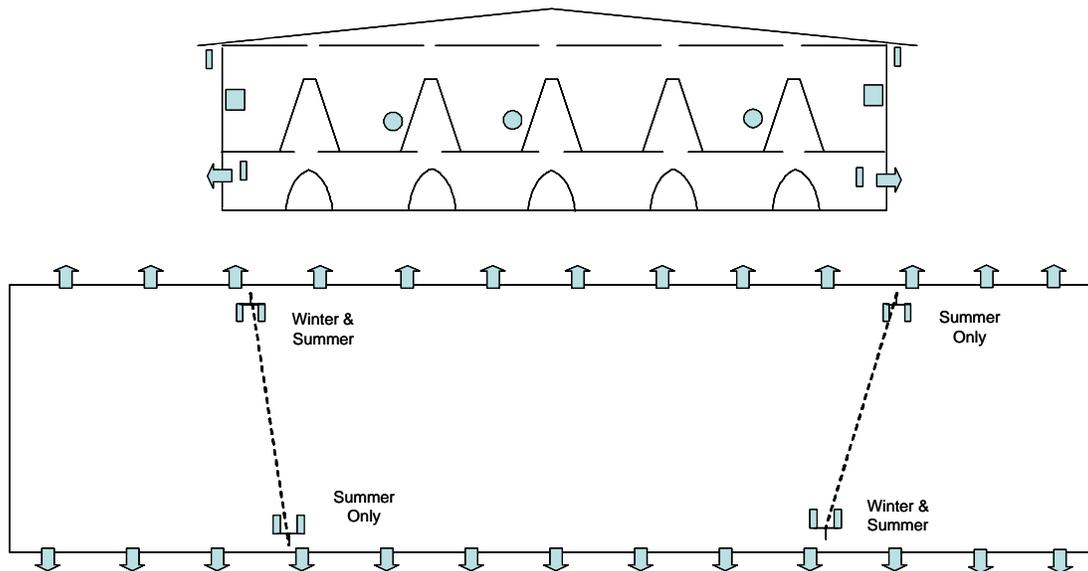
Figure 3. Schematic layout of the IA high-rise layer house showing the cross-section and floor plan of the house and the sampling locations (symbols are the same as in fig. 1).
