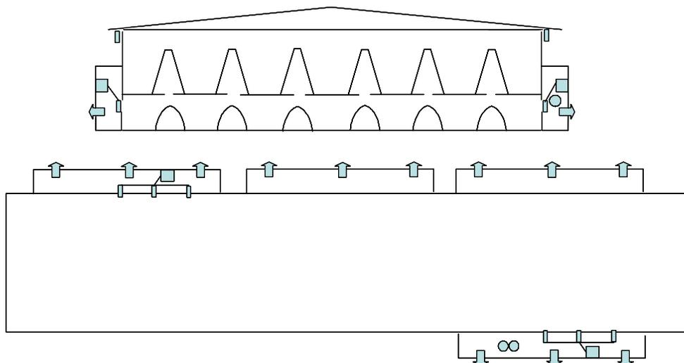
Figure 4. Schematic layout of the PA high-rise layer house showing the cross-section and floor plan of the house and the sampling locations (symbols are the same as in fig. 1).
