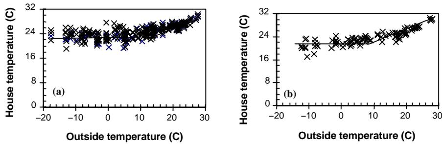
Figure 5. Daily mean air temperature versus daily mean outside temperature in (a) manure-belt and (b) high-rise IA layer houses.
