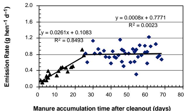
Figure 11. Ammonia emission vs. time of manure accumulation after cleanout in four high-rise houses in IA.
