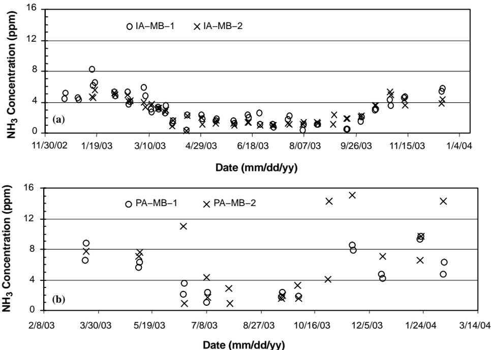
Figure 6. Daily mean ammonia concentrations in exhaust air of manure-belt layer houses in (a) IA and (b) PA.
