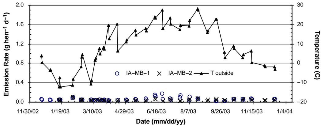
Figure 9a. Daily mean ammonia emission from manure-belt layer houses in IA, where manure was removed from the houses daily, and outside temperature.
