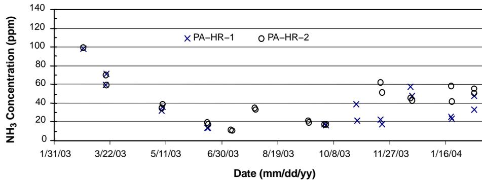
Figure 7b. Daily mean ammonia concentrations measured at exhaust fans of high-rise (HR) layer houses in PA.
