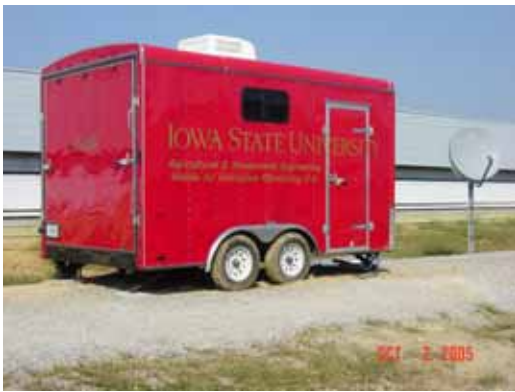
Figure 1: Mobile air emissions monitoring unit on site at a Tyson Foods broiler house. The mobile lab houses the data acquisition system used for the Tyson study.
