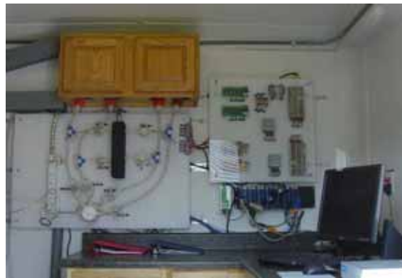
Figure 1: Mobile air emissions monitoring unit on site at a Tyson Foods broiler house. The mobile lab houses the data acquisition system used for the Tyson study.
