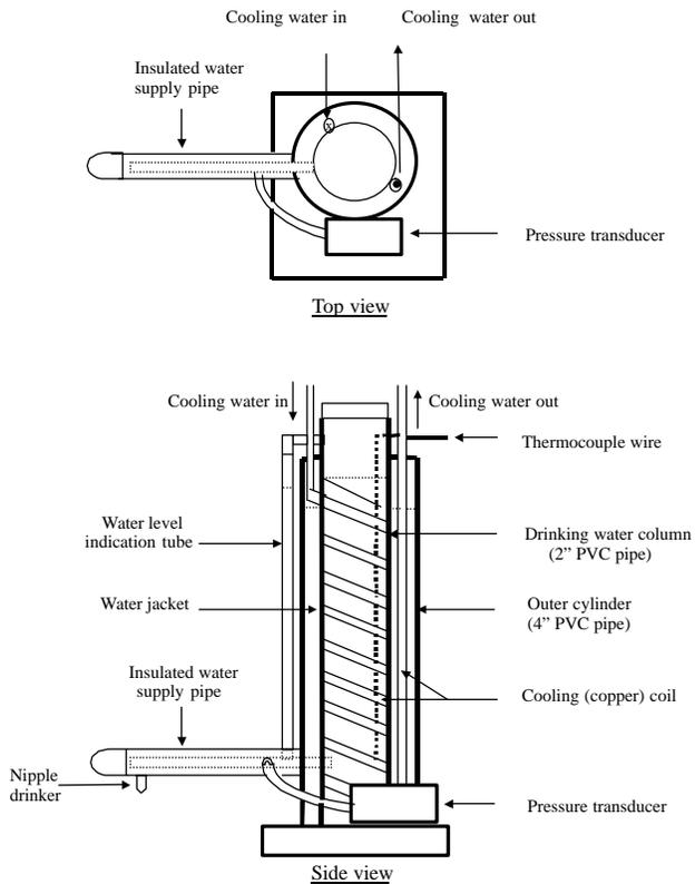
**Figure 2.** Schematic representation of the modified watering unit (not drawn to scale).
