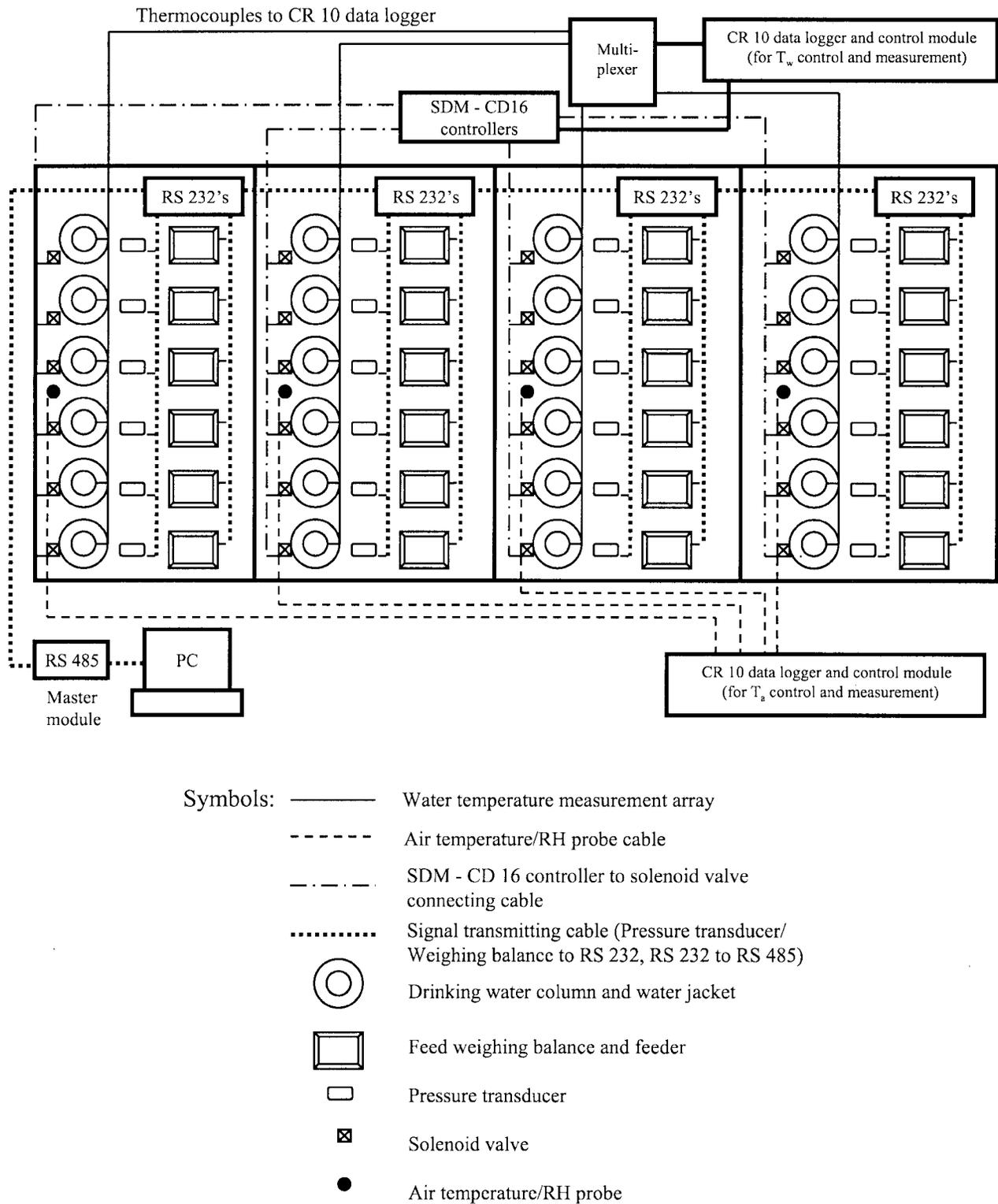
Figure 3. Schematic wiring connections of the measurement and control system for studying feeding and drinking behaviors of individual poultry (not drawn to scale).
