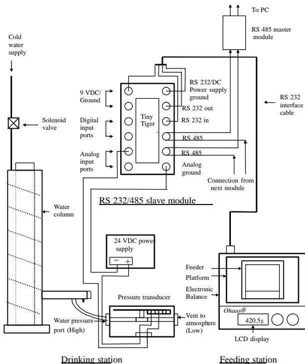
Figure 1. Schematic configuration of individual feeding and drinking station and connections to RS232/485 slave communication module (not drawn to scale).
