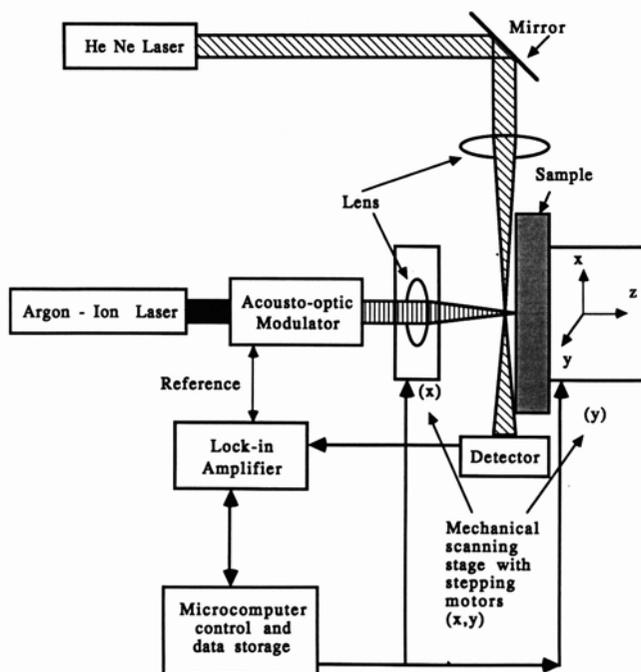
Fig. 3 Block diagram of the mirage effect method for thermal wave imaging.
