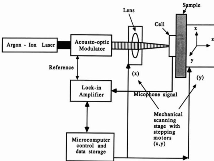
Fig. 1 Block diagram of the gas-cell method for thermal wave imaging.
