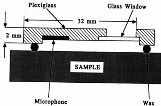
Fig. 2 Schematic diagram of the gas cell.
