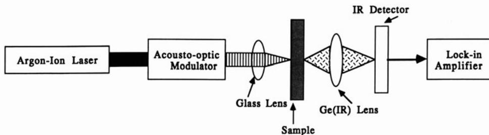
Fig. 4 Block diagram of the photothermal radiometric method for thermal wave imaging.
