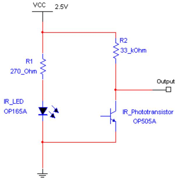
Figure 1. Circuit diagram of infrared emitter detector pairs used to detect bird presence at a feeder opening.
