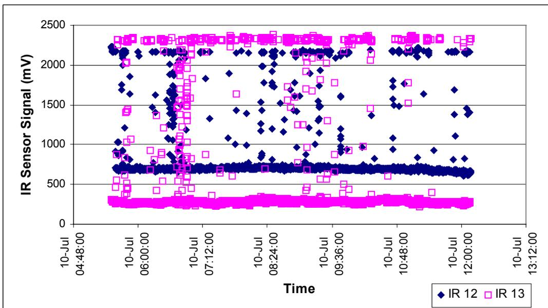
Figure 4. Sample of two raw infrared sensor signals used to determine the presence of a hen at a particular feeder opening.
