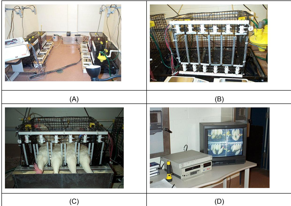
Figure 2. Photo views of the experimental setup: testing room (A); close-up view of feeder access openings with IR sensor pairs above and below each opening (B); hens feeding through instrumented feeder openings (C); video display and recording system (D).
