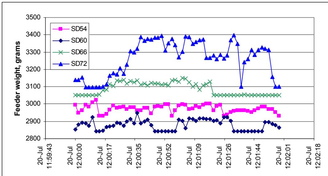
Figure 3. Two-minute time series of raw feeding event signals from the electronic balances of different stocking density (SD) indicating the dynamic feeder weight in grams.
