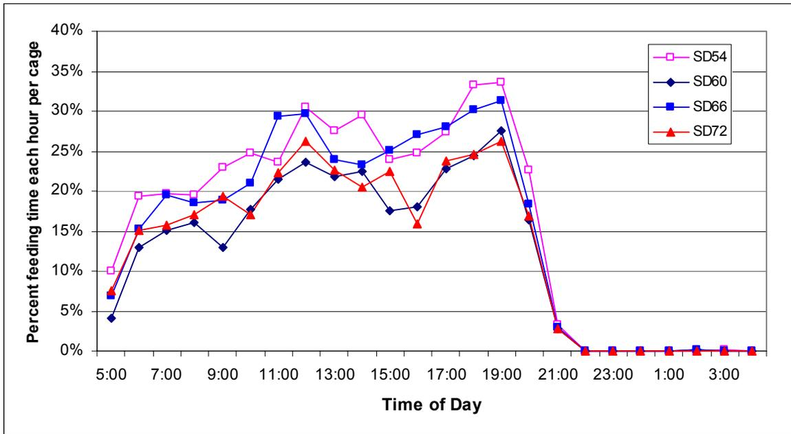
Figure 5. Diurnal feeding patterns of hens at four stocking densities (348, 387, 426, and 465 cm<sup>2</sup> per hen; 54, 60, 66, and 72 in<sup>2</sup> per hen). Chart displays average percent of time spent feeding in each hour. Based on averages from four days' feeding data from each group of 24 hens. Lighting schedule was 16h light (5:30AM-9:30PM) and 8h dark (9:30PM-5:30AM). Data for Group 1 of SD54 were omitted due to mortality.
