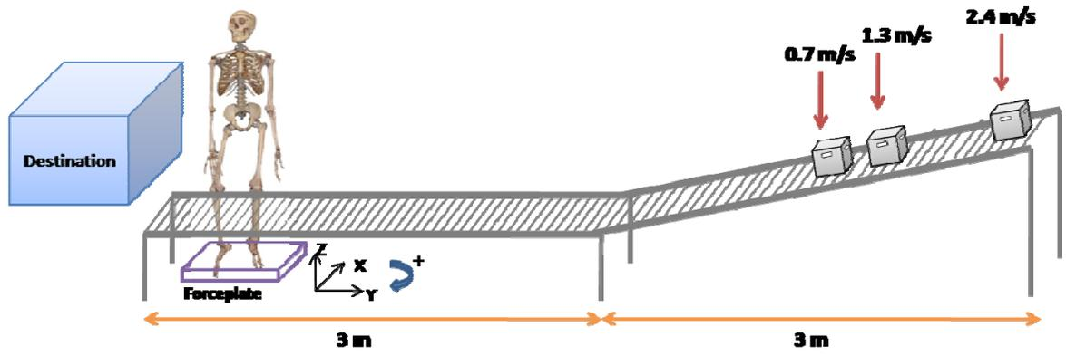
Figure 1. Experimental setup for the conveyor lifting task
