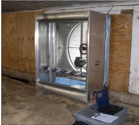
Upstream placement of FANS at the turkey site
