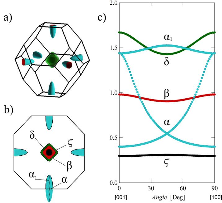
Figure 3: (Color online) (a) Fermi surface (b) sketch through the Brillouin zone of a (001) of YAs calculated in this work using FP-LAPW method with spin-orbit coupling. Triplicate electron pocket and three hole pockets labeled  $\alpha$ ,  $\beta$ ,  $\delta$  and  $\zeta$ . (c) The corresponding (110)-plane angle evolution of the cross-sectional areas (in frequency units) of the calculated Fermi surface pockets.
