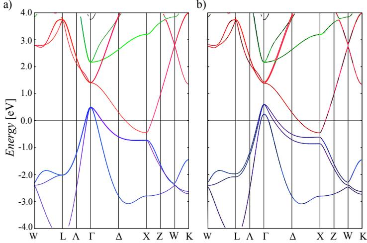
Figure 2: (Color online) Energy bands dispersion in YAs calculated using scalar relativistic FP-LAPW method without (a) and with (b) inclusion of SO coupling. The amounts of Y- $d$  and As- $p$  characters are indicated by the colors of the bands: green symbols denote Y- $d - e_g$ , red Y- $d - t_{2g}$ , and blue As- $5p$ , respectively.
