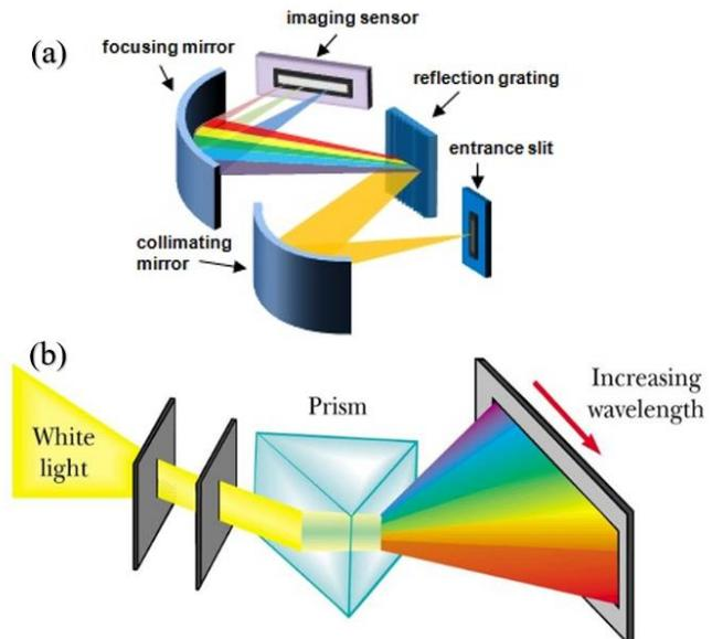
Fig. 1 Two types of transitional optical spectrometers using light refraction: (a) the structure of the optical spectrometer using grating [1]; (b) the structure of the optical spectrometer using prism [2].
