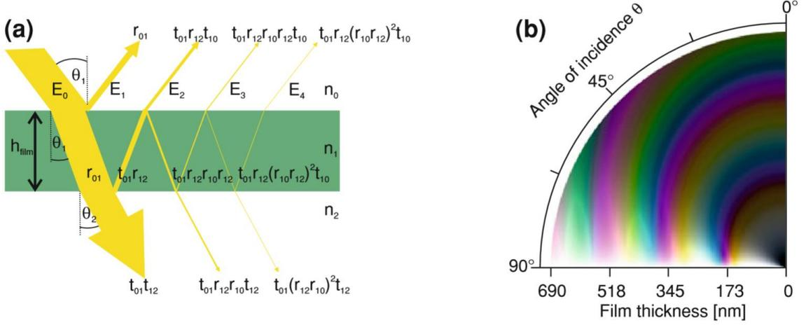
Fig. 4 Thin film interference [4]: (a) reflection and refraction model of the thin film interference; (b) illustration of the color reflection of a thin film plotted by computer-simulation
