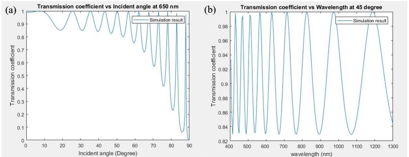
Fig. 5 Results of the thin film interference simulation in MATLAB: (a) plot of transmission coefficient vs incident angle at 650 nm; (b) plot of transmission coefficient vs wavelength at 45 degree of incident angle
