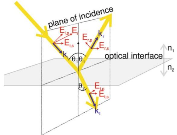
Fig. 3 The diagram of reflection and refraction at an optical interface [4]
