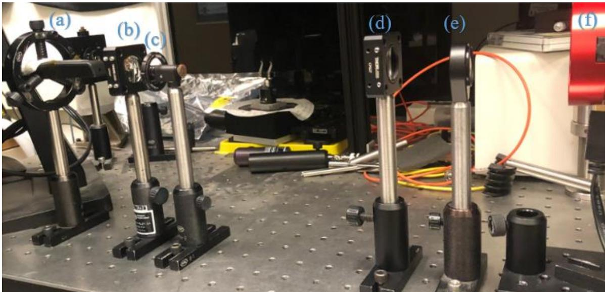
Fig. 10 The setup of the compact spectrometer. From left to right: (a) red light laser pointer; (b) convex lens; (c) optical filter; (d) cylindrical lens; (e) convex lens; (f) CMOS camera
