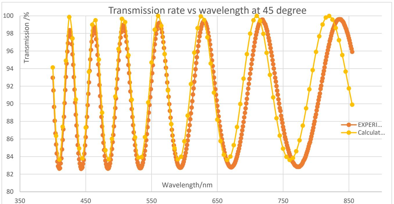
Fig. 6 Comparison of the simulated transmission vs wavelength plot in Excel and the measured one from Thorlabs [5] at 45 degree of incident angle. In the simulation, the refractive index keeps the same as 1.5 and there is an assumption of no absorption on the thin film.
