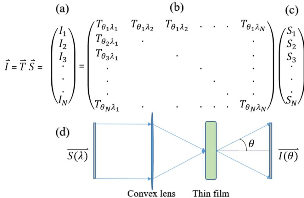
Fig. 7 Explanation of using transmission matrix of the thin film and detected light intensity on CMOS camera to find out the spectrum of the input optical signal: (a) matrix of measured intensity on CMOS camera  $\vec{I}$ ; (b) transmission matrix of the thin film; (c) matrix of the unknown input light spectrum; (d) diagram of the light propagation in the spectrometer
