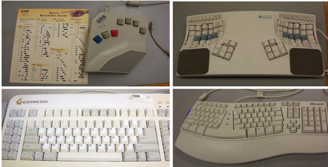
Figure 1: The four alternative keyboards used in this study: chord (top left), contoured split (top right), Dvorak (bottom left), split fixed-angle (bottom right).
