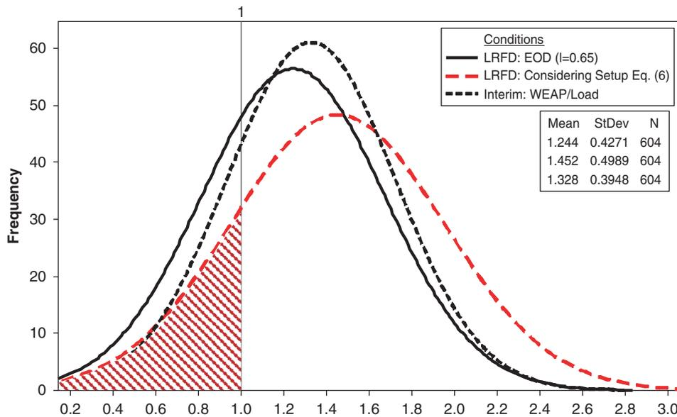
FIGURE 3 Ratio of driving resistance to target resistance or bearing [LRFD (EOD) = ratio of measured driving resistance at EOD to target driving resistance ( $\gamma Q/\varphi_{EOD}$ ); LRFD (considering setup) = ratio of measured driving resistance at EOD to target driving resistance (Equation 6); Interim = ratio of driving resistance (considering safety factor = 2.2) to service load (plan design bearing)].
