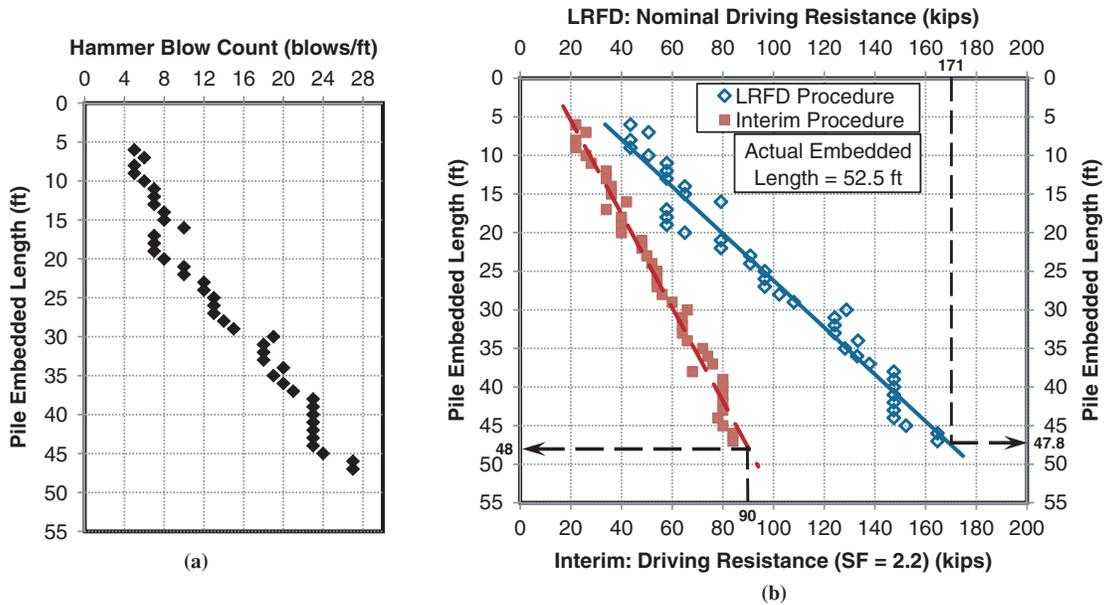
FIGURE 4 Driving details of Production Pile 8 at Pier 1 in Cedar County, Iowa: (a) detailed pile-driving record and (b) detailed pile-driving resistance graph (SF = safety factor).
