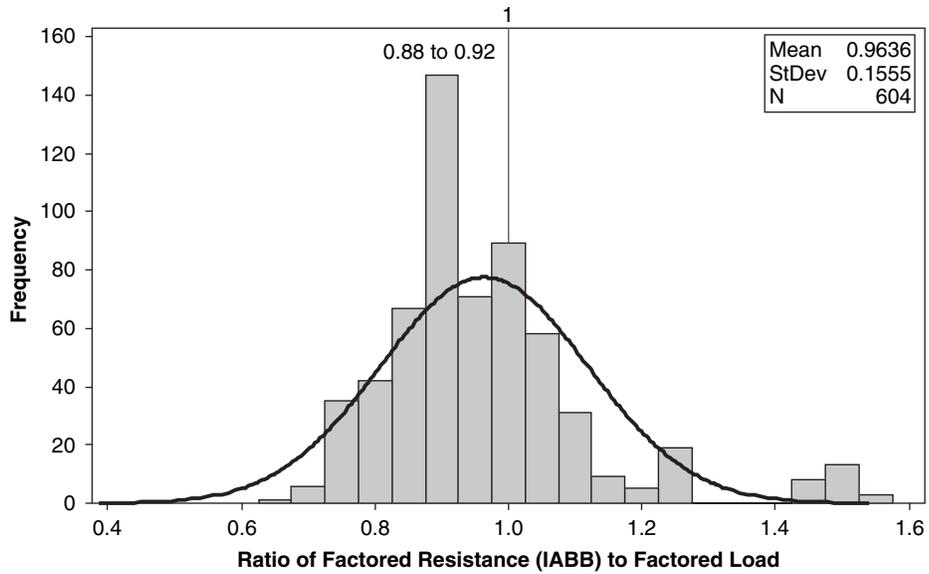
FIGURE 1 Ratio of factored geotechnical resistance, estimated with IABB, to factored applied load (StDev = standard deviation).
