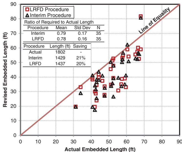
FIGURE 5 Comparison of required embedded pile lengths for interim and LRFD procedures and actual embedded pile lengths.
