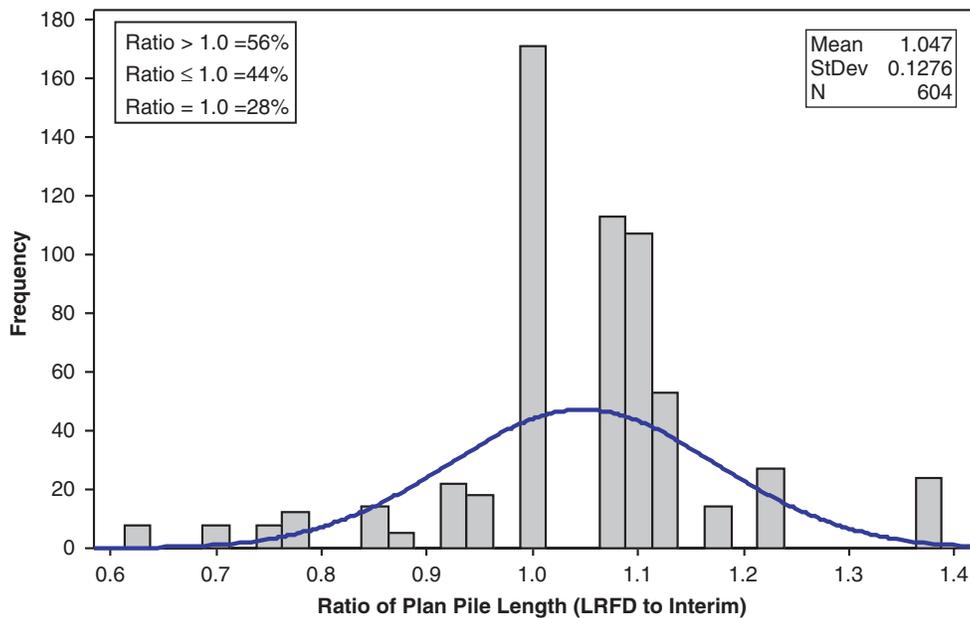
FIGURE 2 Comparison of plan pile lengths estimated with LRFD procedure and interim procedure.
