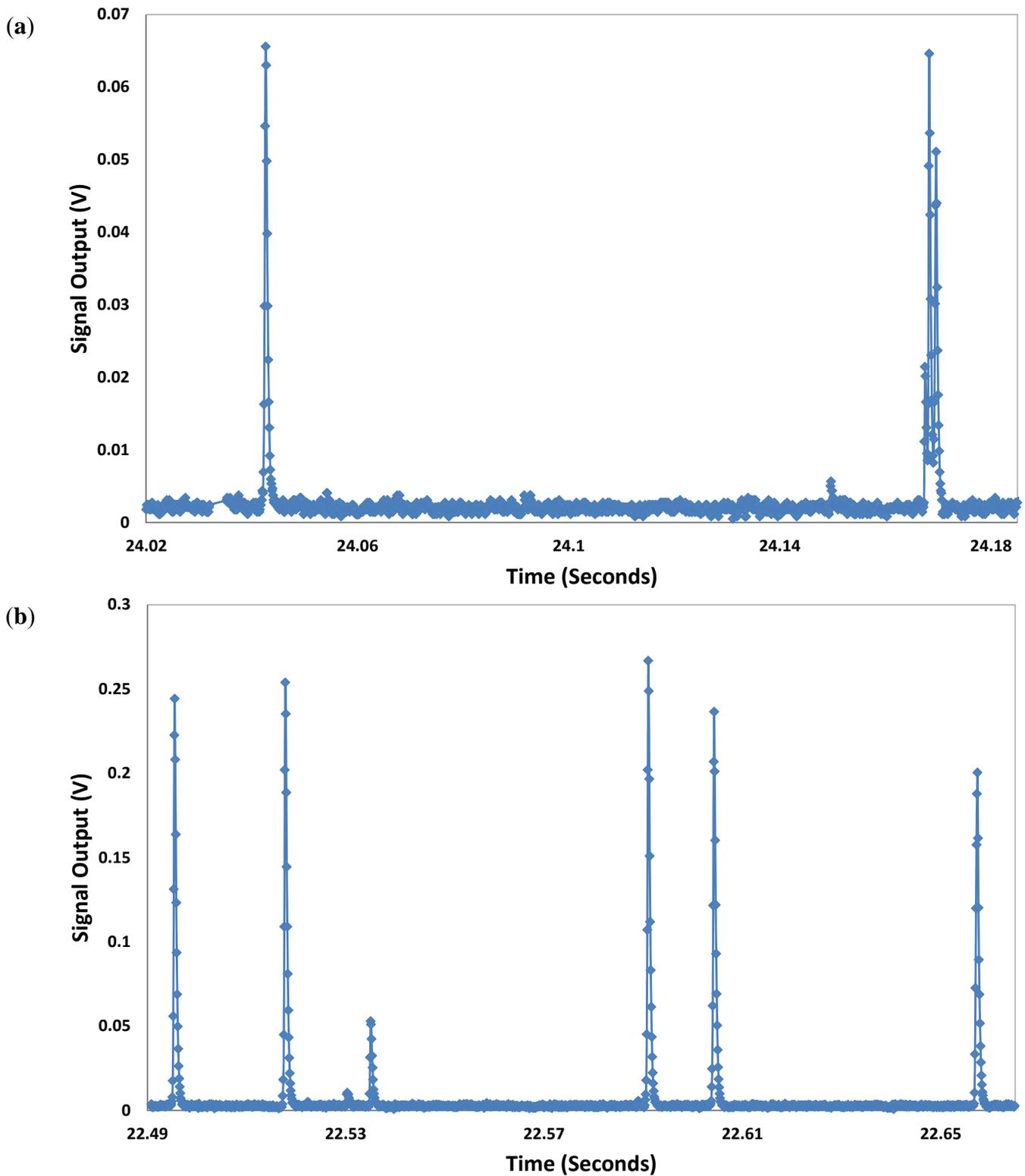
**Figure 3.** Voltage outputs produced by the (a) 3.2 μm and (b) 10.2 μm beads and collected by the MPPC. The signals collected for the 10.2 μm bead showed higher amplitude and width compared to those of the 3.2 μm bead. The 35 mW diode laser was used for excitation.
