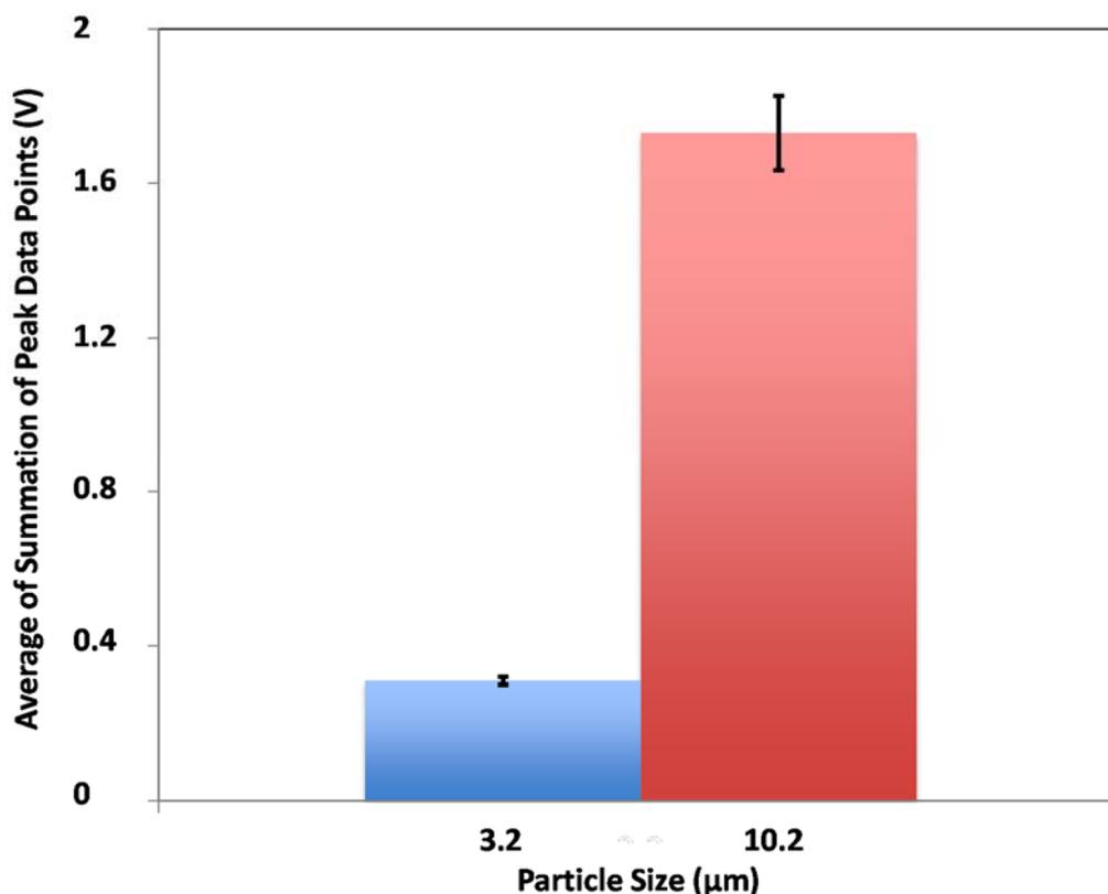
**Figure 4.** The statistical analysis for two different sizes of beads. The red bar shows higher average value for the summation of peak data points (SPDPs) for 10.2 μm particles compared to the average value calculated for 3.2 μm particles (blue bar). The average of SPDPs is 0.31 V for 3.2 μm and 1.71 V for 10.2 μm. The standard deviation is shown on each column.
