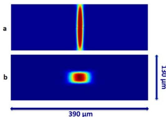
**Figure 2.** The concentration distribution along the channel for the cross section at: (a) before the arrays of chevrons; (b) after the fourth chevron groove. The sheath stream focuses the core stream vertically before the chevrons. As the flow passes through the chevrons, the sheath stream focus the core stream horizontally in the middle of the channel. The concentration of sheath and sample streams were assumed to be  $0 \text{ mol}/\text{m}^3$  (blue) and  $1 \text{ mol}/\text{m}^3$  (red).
