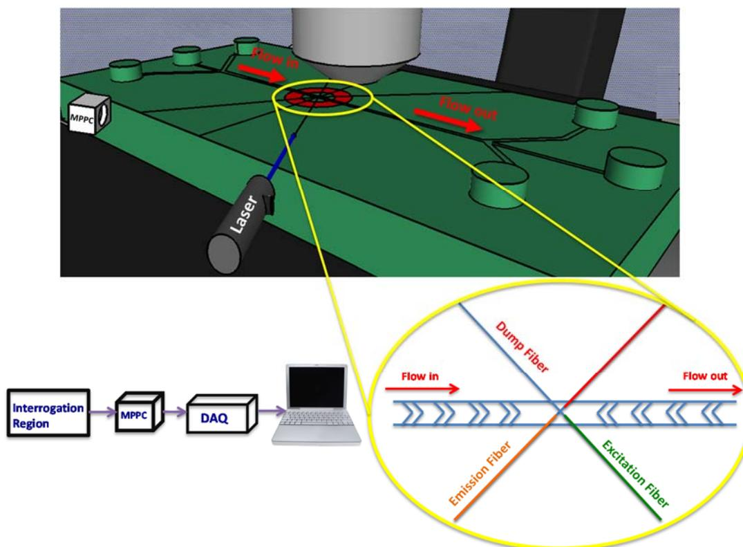
**Figure 1.** A schematic of the microfluidic chip with integrated optics. The laser beam is transferred through a fiber to the interrogation region where the microparticles pass through. An multi-pixel photon counter (MPPC) collects scattered light from the microparticles transferred by the emission fiber. A data acquisition unit collects the analog data from the photodetector and sends it to a desktop computer for further analysis.
