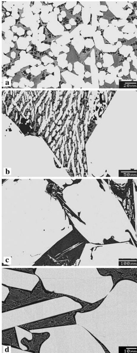
Fig. 4—SEM images showing observed microstructures after heat treating the as-arc-melted Al-18 at. pct Sm alloy at (a) 973 K for 22 h, (b) 1173 K for 25 h, (c) 1293 K for 22 h, and (d) 1373 K for 25 h (each followed by water quenching).
