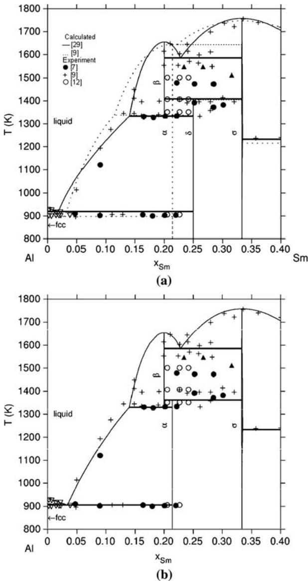
Fig. 1—(a) Al-Sm phase diagram. (b) The metastable Al-Sm phase diagram (with the  $\delta$  phase suppressed).
