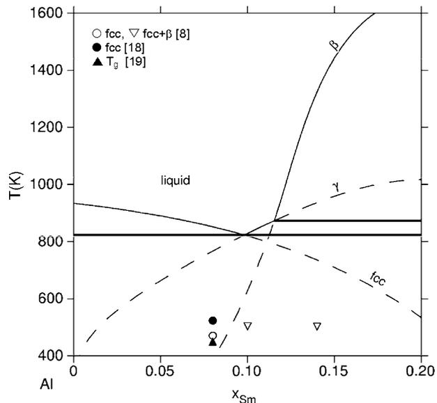
Fig. 7—Metastable liquidus curves for the indicated phases.
