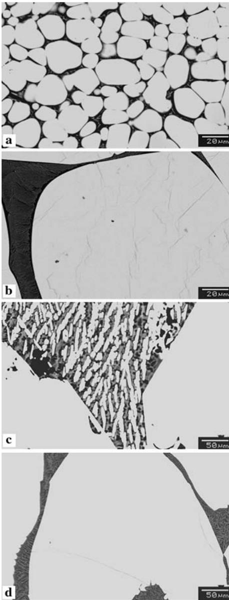
Fig. 2—SEM images showing observed microstructures after heat treating the as-arc-melted Al-18 at. pct Sm alloy at 1173 K for (a) 0 h, (b) 21 h, (c) 25 h, and (d) 46 h (each followed by water quenching).
