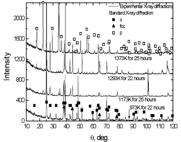
Fig. 5—XRD data for the alloys shown in Fig. 4.
