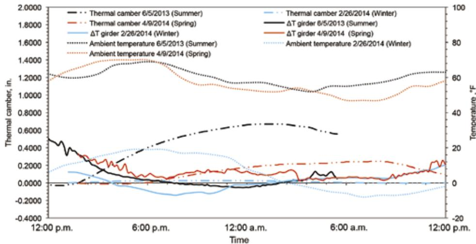
**Figure 1.** Variation of measured thermal camber, ambient air temperature, and the girder temperature difference between the top and bottom flange surfaces for a BTE145 girder. Note:  $\Delta T$  = temperature difference over the height of the girder. 1 in. = 25.4 mm;  $^{\circ}\text{C} = (^{\circ}\text{F} - 32)/1.8$ .
