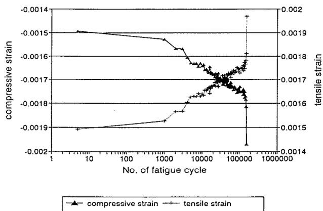
FIG. 1. Maximum tensile and compressive strain as a function of number of stress cycles at a fixed stress amplitude of 272 MPa.
