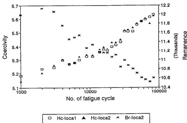
FIG. 3. Magnetic properties as a function of the number of stress cycles.
