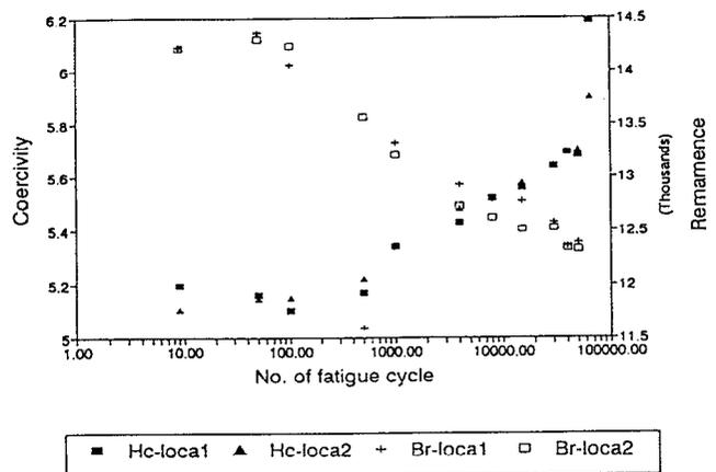
FIG. 4. Magnetic properties as a function of the number of stress cycles.
