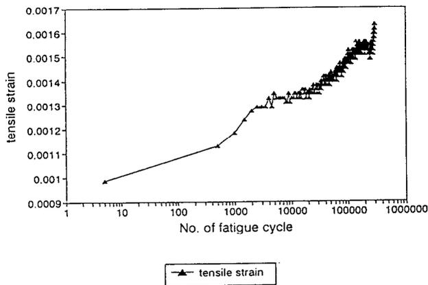
FIG. 2. Maximum tensile strain as a function of number of stress cycles at a fixed stress amplitude of 243 MPa.
