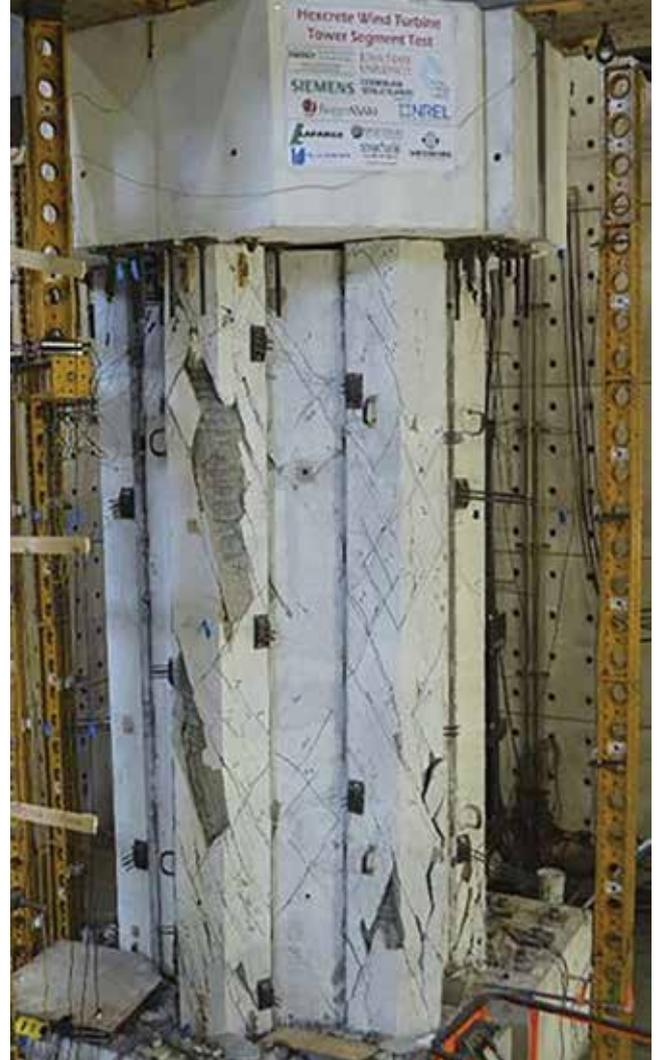
**Figure 6.** This full-scale Hexcrete cell, which would be located near the top of a 394 ft (120 m) tall tower, has been assembled and subjected to a variety of loads representing operational, extreme, and ultimate limit states.
