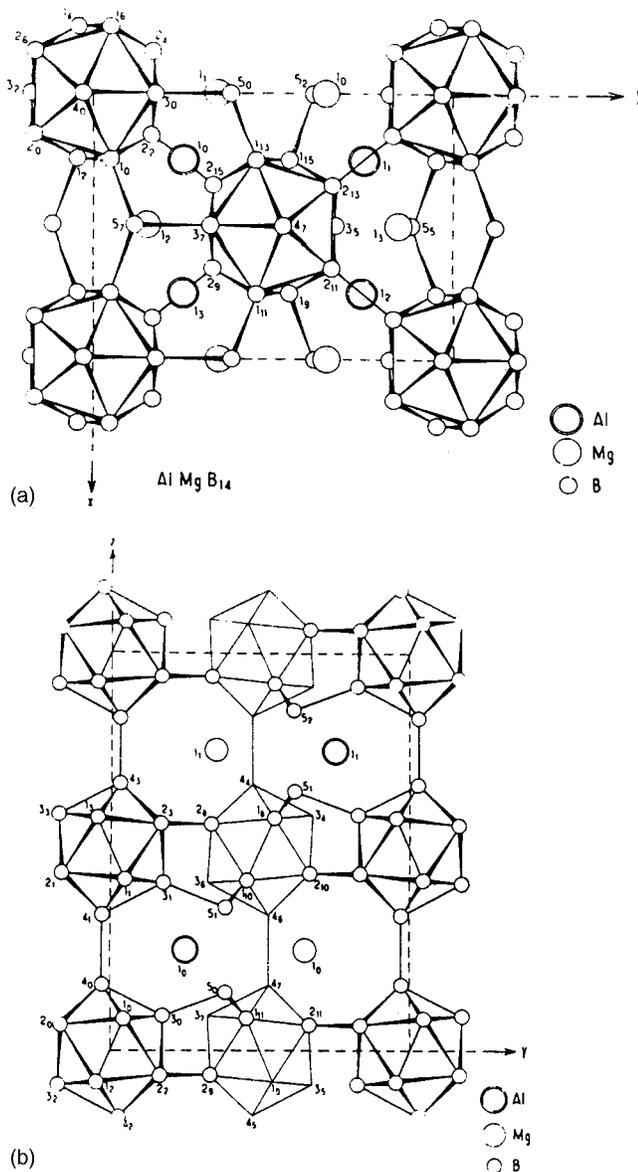
FIG. 1. Crystal structure of orthorhombic  $\text{AlMgB}_{14}$ . (a) Projection on the  $ab$  plane. (b) Projection on the  $bc$  plane.
