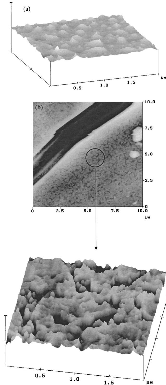
FIG. 5. (a) AFM images of the room-temperature-as deposited  $\text{AlMgB}_{14}$  film. (b) AFM images of the room-temperature-deposited, 1273 K-annealed  $\text{AlMgB}_{14}$  film.
