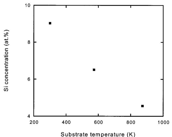
FIG. 2. Relation between Si concentration (at. %) in the 1273 K-annealed films and substrate temperatures during film deposition.
