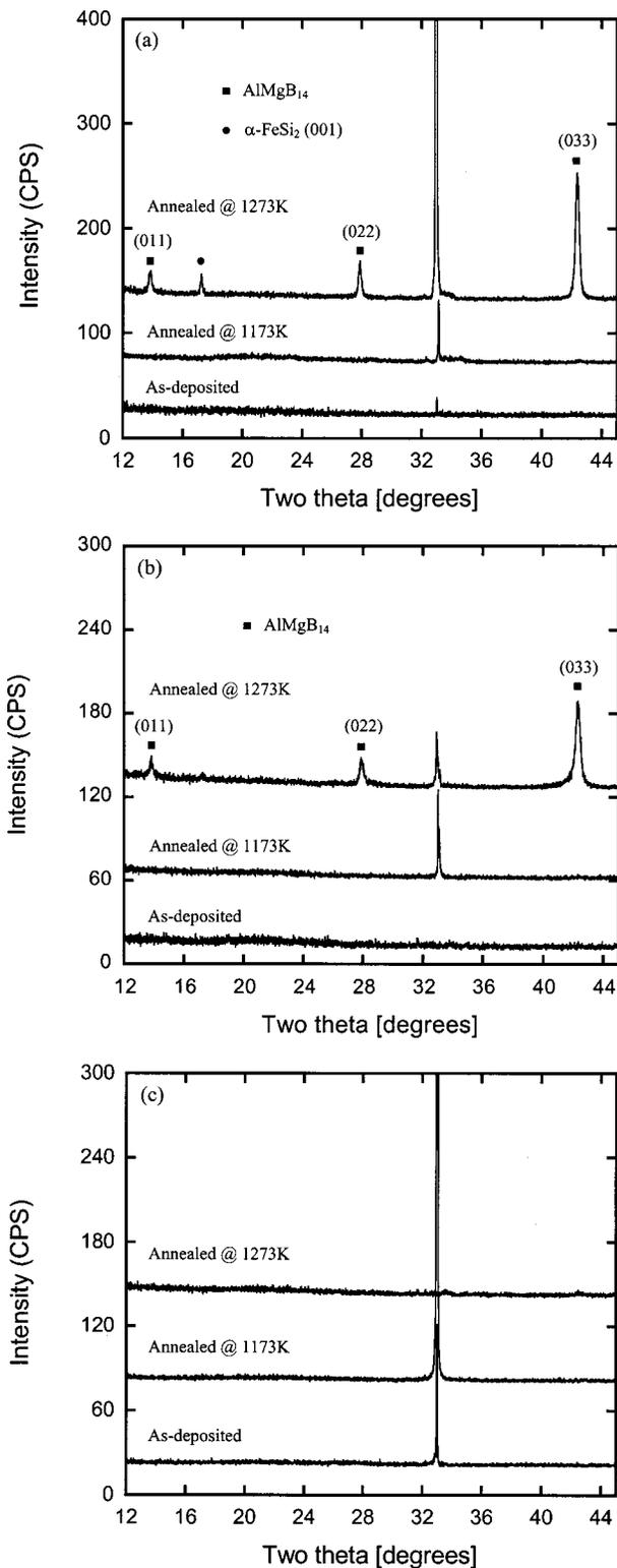
FIG. 3. (a) XRD patterns for the room-temperature as-deposited film, the room-temperature-deposited 1173 K-annealed film and the room-temperature-deposited 1273 K-annealed film. (b) XRD patterns for the 573 K as-deposited film, the 573 K-deposited 1173 K-annealed film, and the 573 K-deposited 1273 K-annealed film. (c) XRD patterns for the 873 K as-deposited film, the 873 K-deposited 1173 K-annealed film, and the 873 K-deposited 1273 K-annealed film.
