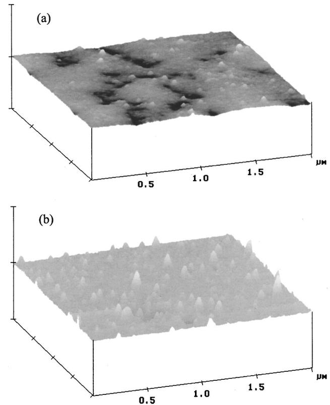
FIG. 6. (a) AFM images of the 573 K-as deposited  $\text{AlMgB}_{14}$  film. (b) AFM images of the 573 K-deposited, 1273 K-annealed  $\text{AlMgB}_{14}$  film.
