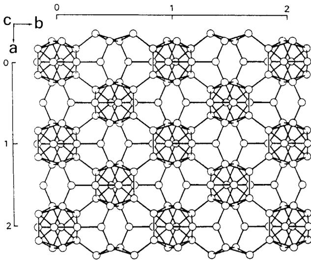
FIG. 4. Icosahedral  $B_{12}$  network parallel to the (001) plane of orthorhombic  $AlMgB_{14}$  (see Ref. 35).
