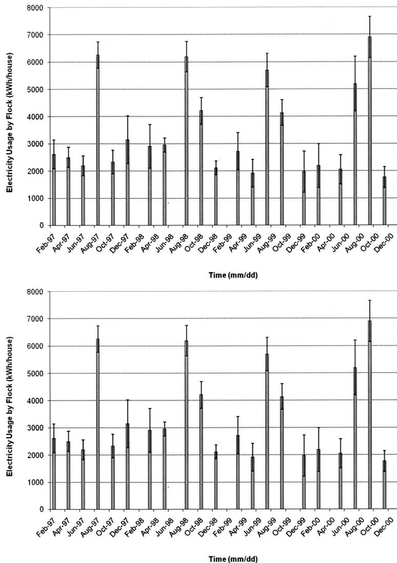
**Figure 1. Total average electricity usage pooled over the four broiler houses (18,000 to 19,500 straight-run broilers per house) for flocks between years 1997 and 2000. Error bars represent standard deviation of the four houses. (a) Electricity use by house; (b) Electricity use by 1000-kg market weight.**
