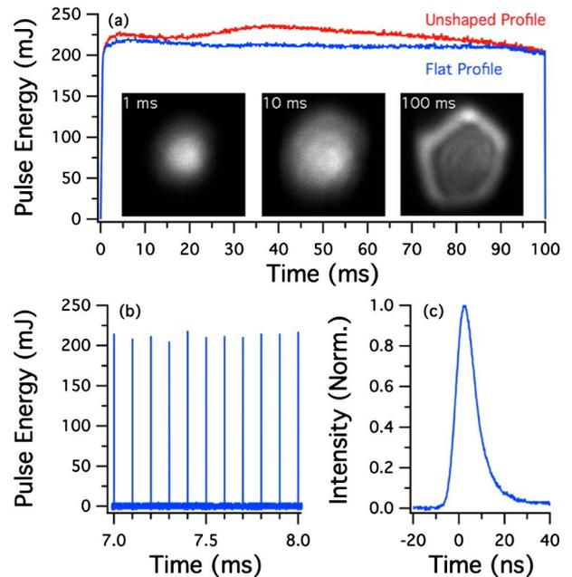
Fig. 4. (a) Comparison of unshaped and flat-top burst-profile pulse energies over 100 ms. (b) 1 ms segment of (a) showing 10 kHz operation, and (c) profile of an individual pulse with pulse width of 9.85 ns (FWHM).
