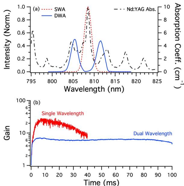
Fig. 2. (a) Comparison of single-wavelength array (SWA) and dual-wavelength array (DWA) diode emission relative to 808 nm Nd:YAG absorption [15], and (b) time-dependent small-signal gain of 5 mm SWA and DWA amplifiers.
