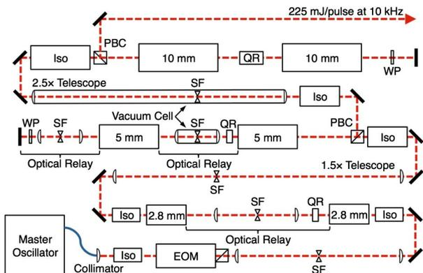
Fig. 1. Schematic of 100 ms, all-diode-pumped burst-mode laser system. Dashed line represents beam pathway through system. Diode amplifiers are listed by rod diameter. Iso, optical isolator; EOM, electro-optic modulator; SF, spatial filter; QR, quartz rotator; PBC, polarizing beam cube; WP, quarter-wave plate.
