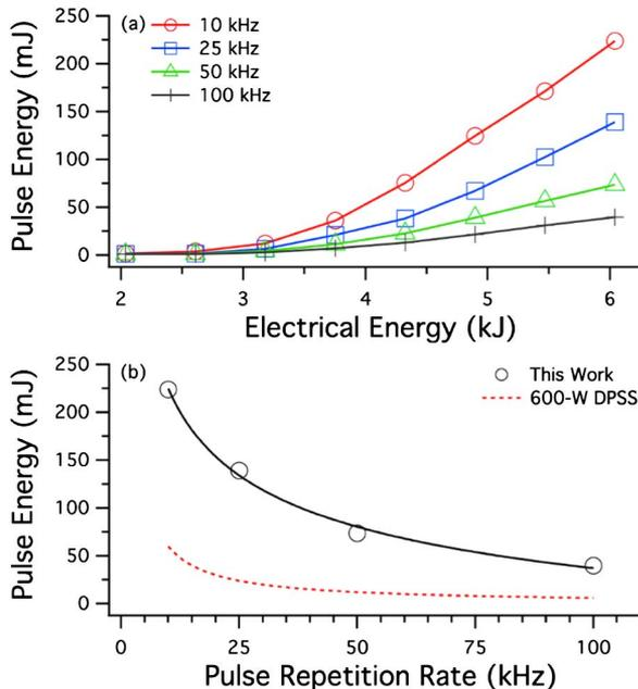
Fig. 3. Individual pulse energy as a function of (a) total electrical energy delivered to the system and (b) pulse repetition rate. Burst-to-burst standard deviation of 0.8% falls within the symbol size. The experimental data is fit to a power law scaling and compared with the calculated performance of a 600 W DPSS laser [3].
