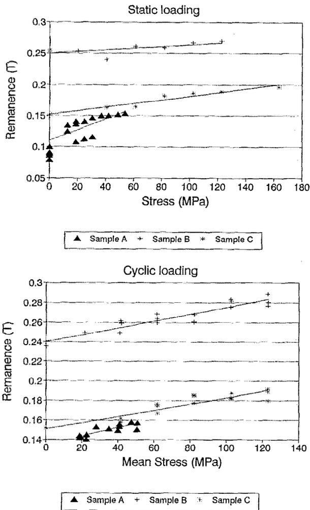
FIG. 4. Remanences measurements on samples of steel bridge material subjected to (a) static loading and (b) cyclic loading.
