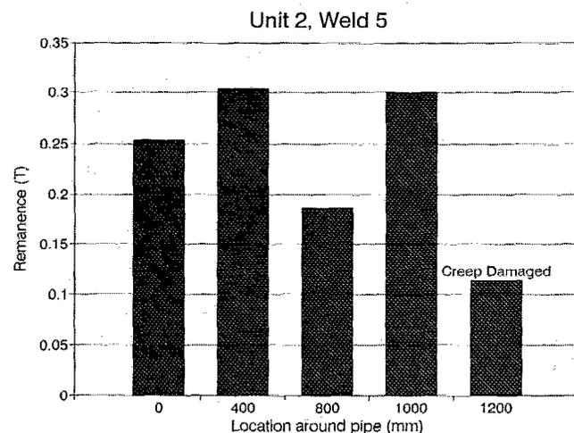
FIG. 1. Remanence measurements around the diameter of creep damaged pipeline of diameter 1600 mm. Creep damage was identified at a location corresponding to 1200 mm around the diameter. This can be seen to correspond to a low remanence.
