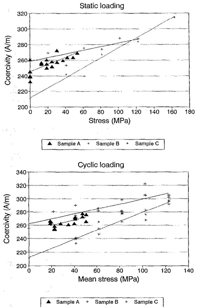
FIG. 3. Coercivity measurements on samples of steel bridge material subjected to (a) static loading and (b) cyclic loading.
