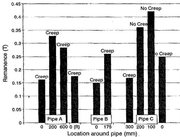
FIG. 2. Remanence measurements on welds of three creep damaged pipe-lines. The remanence at creep damaged locations was generally smaller than the remanence at most of the undamaged locations.
