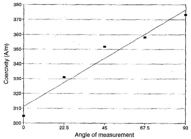
FIG. 5. Coercivity measured with respect to angle for service aged Cr-Mo steel.
