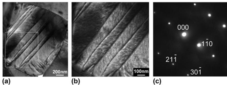
FIG. 1. (a) Bright-field micrograph of a representative grain along its [113] zone axis in the virgin state of 0.7PMN-0.3PT ceramic. (b) Higher magnification image of the boxed area in (a) to show the hierarchical domain structure. (c) The corresponding selected area diffraction pattern.
