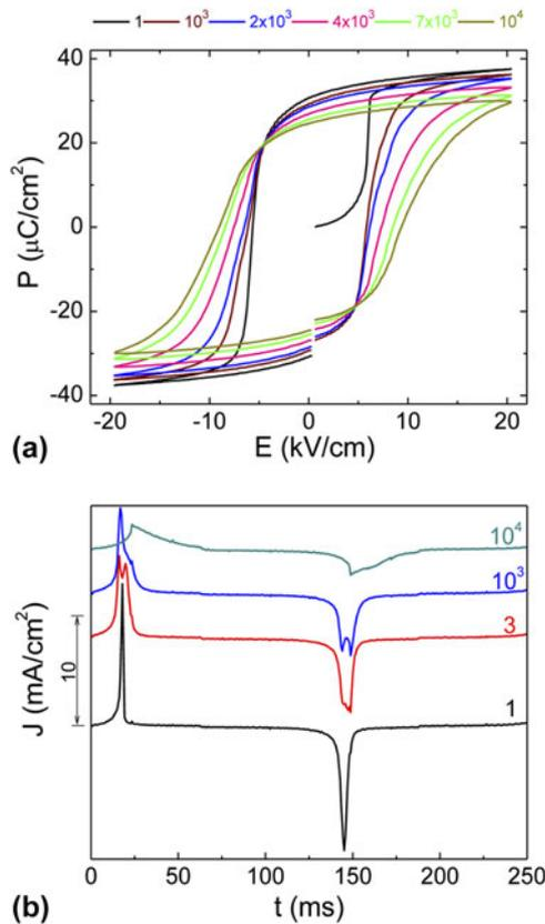
FIG. 4. (a) Change of the polarization hysteresis loop and (b) polarization current density curves during electric fatigue in 0.7PMN-0.3PT bulk ceramic.
