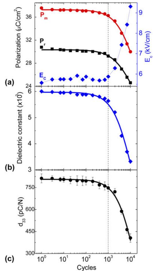
FIG. 5. (a) Polarization and coercive field, (b) dielectric constant, and (c) piezoelectric coefficient as a function of cycling number measured from the same bulk specimen as in Fig. 4. The experimentally measured results are shown as discrete points, while the solid fitting curves are derived using the power-law relation. The fitting equations are shown in the text.
