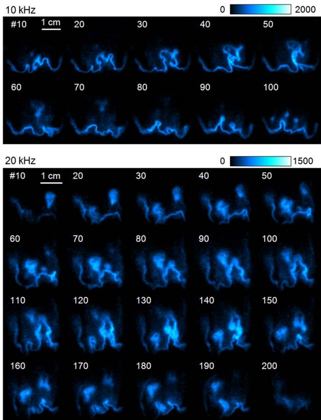
Fig. 4. (Color online) 10 ms duration PLIF imaging of  $\text{CH}_2\text{O}$  in a lifted  $\text{CH}_4$ -air diffusion flame at 10 kHz (upper panel) and 20 kHz (lower panel) showing every 10th image. False-color scales indicate non-normalized, background-subtracted camera counts. The full sequences for 10 kHz and 20 kHz are available online as [Media 1](#) and [Media 2](#), respectively.
