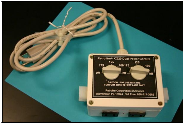
Figure 4: Retrolite® CZ20 Dual Power Controller (DPC) with three settings (100W, 125W and 175W) paired with the plastic fixture.
