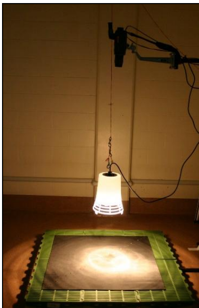
Figure 2: Experimental setup showing the PM250 IR camera above the plastic fixture at 51-cm (20-in) height.
