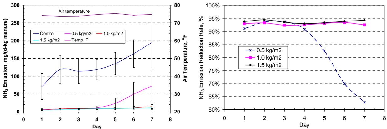
Figure 6. Effect of topical application of alum powder at different rates on ammonia emissions from laying hen manure. The application rates were 0, 0.1, 0.2 or 0.3 lb/ft<sup>2</sup> (0, 0.5, 1.0 or 1.5 kg/m<sup>2</sup>). The vertical bars represent the standard deviations.
