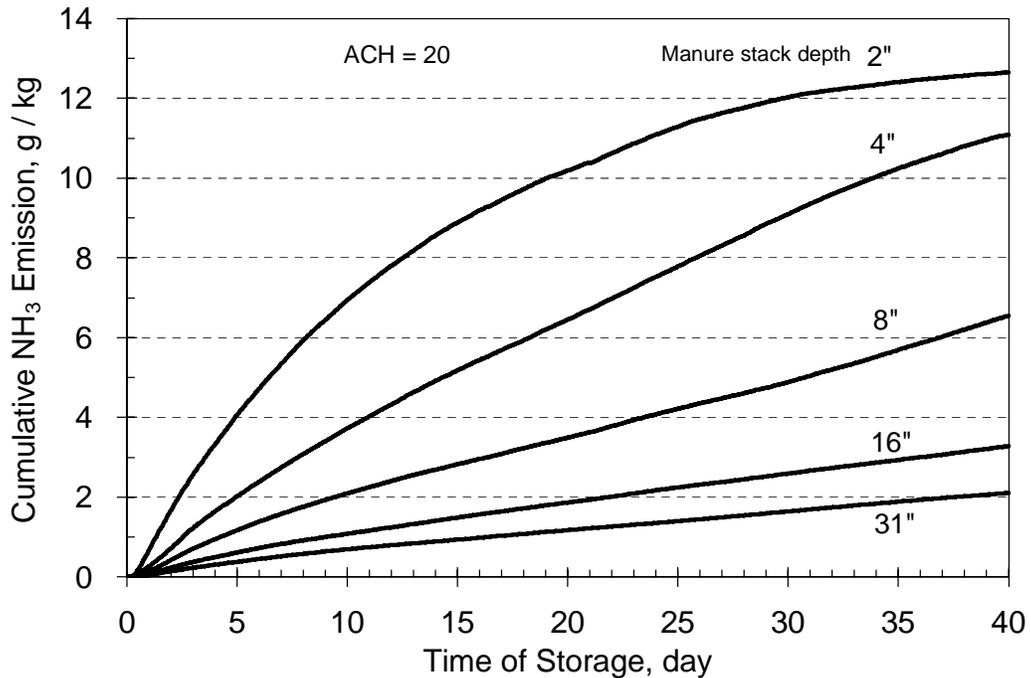
Figure 3. Ammonia emissions from laying hen manure storage as affected by surface area to volume ratio of the manure stack. All stacks had the same base area of 30 ft<sup>2</sup> but with different heights of 2 to 31 inches. Air temperature in all chambers was held at 77°F, with an airflow rate of 20 air changes per hour (ACH).
