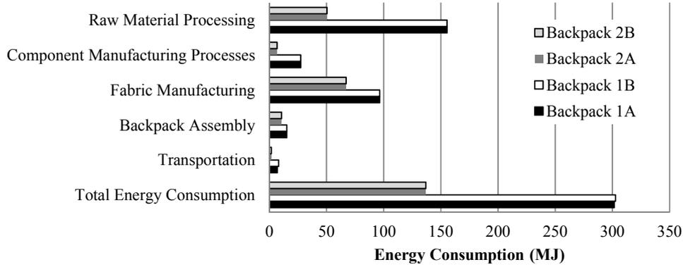
Figure 6 presents a comparison of the energy consumption for the major manufacturing processes for each backpack design. An evident difference between backpacks 1A and 1B are due to transportation energy consumption, which are 6.9 and 8.2 MJ, respectively. For backpack 2, the respective transportation energy consumptions for alternatives A and B are estimated to be 1.87 and 1.74 MJ, respectively. The reduction over backpack 1 is largely due to omission of air transport.
