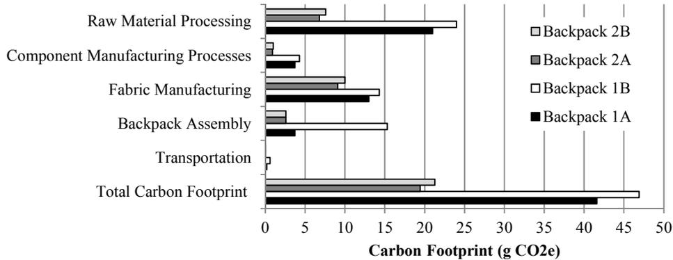
Figure 7 presents the carbon footprint for backpack manufacturing processes and transportation activities for each backpack scenario. Backpack 1B has the largest carbon footprint. For backpack 1A and 1B, the raw material processes dominate the other processes in terms of carbon footprint. For backpack 2A and 2B, however, fabric manufacturing processes have larger carbon footprints than other processes. For each backpack scenario, the carbon footprint of manufacturing dominates that of
