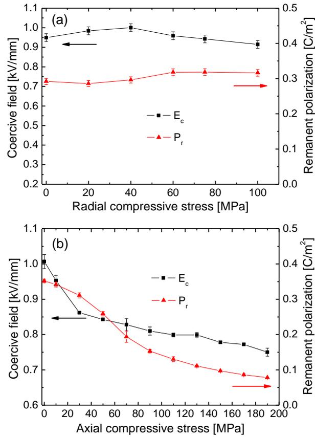
**Figure 5.** Remanent polarization  $P_r$  and coercive field  $E_c$  of a polycrystalline PZT ceramic with tetragonal symmetry under (a) radial, and (b) uniaxial compressive pre-stresses. The data in plot (a) are taken from Reference [21].
