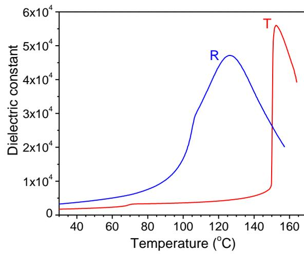
**Figure 1.** Dielectric constant vs. temperature for Crystal R and Crystal T measured at 1 kHz during heating at 3  $^{\circ}\text{C}/\text{min}$ .
