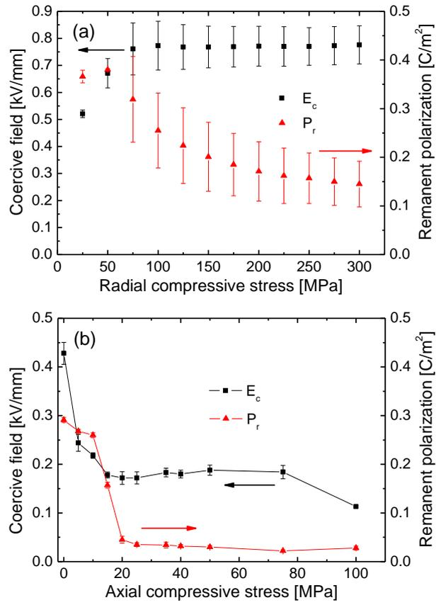
**Figure 4.** Remanent polarization  $P_r$  and coercive field  $E_c$  of Crystal T under (a) radial, and (b) uniaxial compressive pre-stresses.
