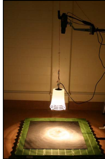
Figure 2: Experimental layout showing the PM250 IR camera above the plastic fixture at 22-inch height.
