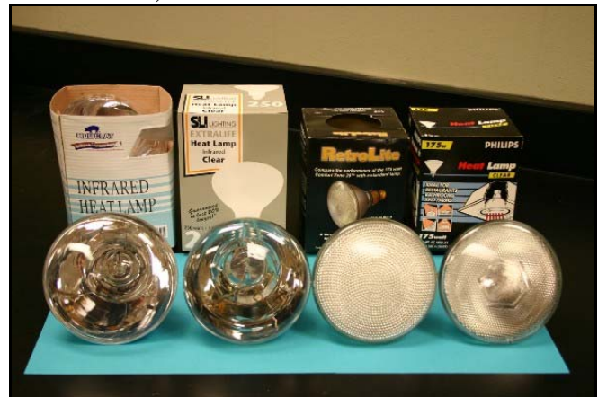
Figure 3: Lamp surface treatment (l to r) for a) 125HOG, b) 125SLI and 250SLI, c) 100SYL and 175SYL and d) 175PLP.
