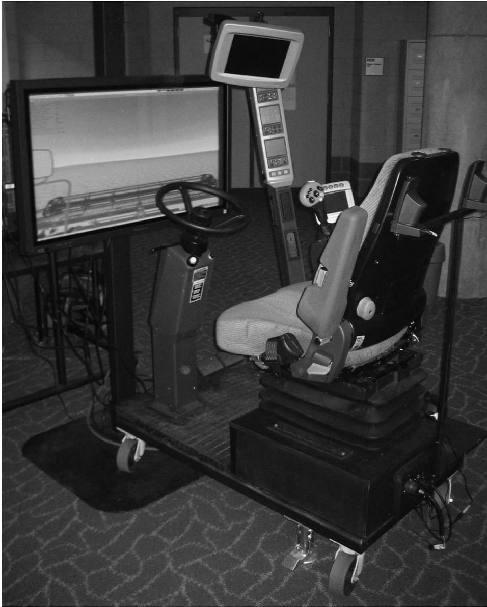
**Figure 5.** *The GREENSPACE stand-alone combine simulator buck at Iowa State University.*
