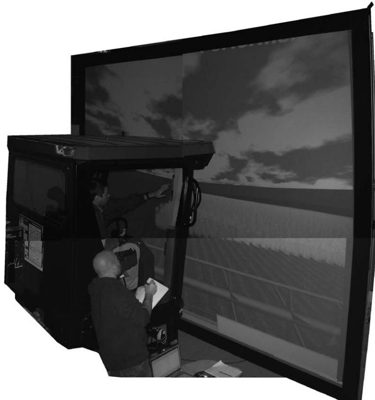
**Figure 2.** Actual operator inputs drive the combine through the virtual farm field.
