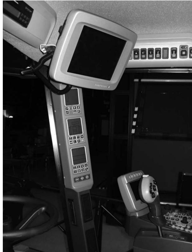
**Figure 4.** The John Deere GS2 CAN controller performs precision farming data integration.
