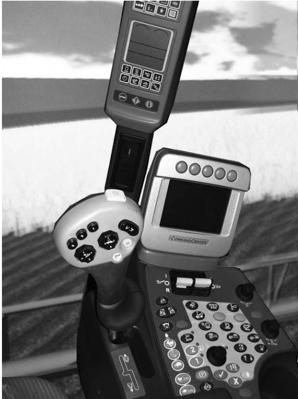
**Figure 3.** The operator drives the simulation with the same controls as the combine. The pair of switches (yellow on the controller) engage the header and reel.
