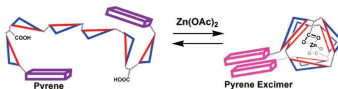
A hybrid foldamer containing six cholate units and two glutamic acids was labeled with two pyrenyl groups at the chain ends. Folding was particularly favorable in the presence of zinc(II), as shown by the enhanced emission of the pyrene excimer. The sensitivity of the detection depended on the relative population of the folded and unfolded conformers, being highest when about 90% of the foldamer was in the unfolded state.
