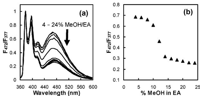
**Figure 2.** (a) Normalized fluorescence spectra of oligomer **1** in different mixtures of methanol and EA. (b) The excimer/monomer ratio ( $F_{472}/F_{377}$ , the emission intensity at 472 nm over that at 377 nm) as a function of solvent composition.
