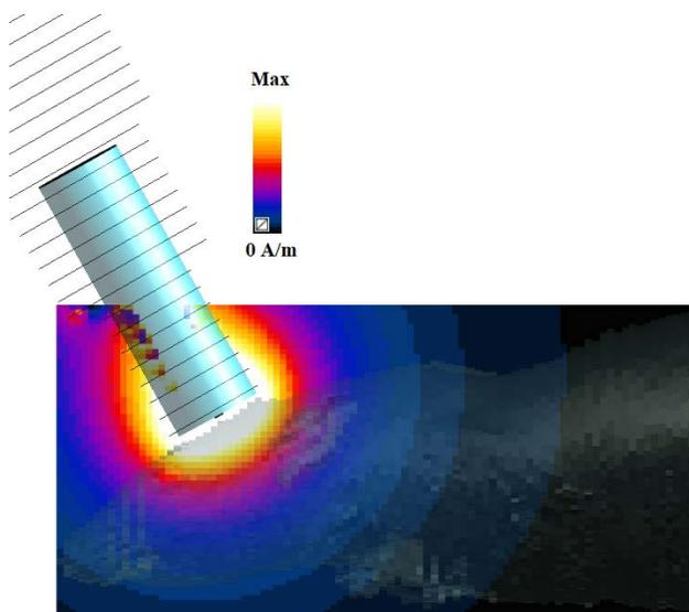
Figure 2. Shows the H-Field profile on a mouse model, maximum H-Field value is 0.5 MA/m.
