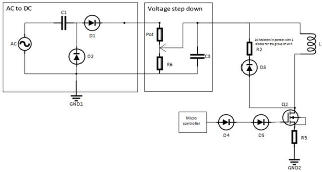
Figure 4. Schematic of a TMS stimulator circuit.
