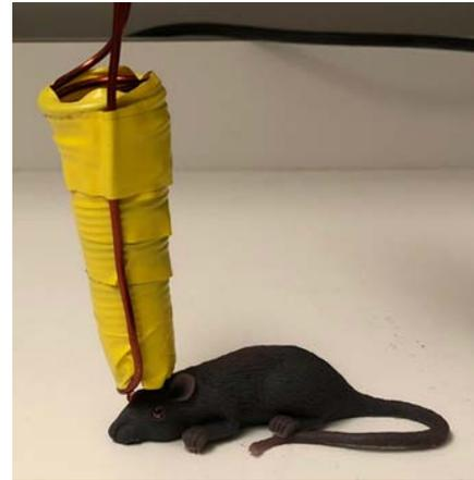
Figure 6. TMS coil is positioned on a plastic mouse model.
