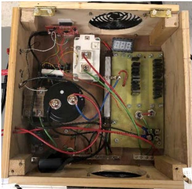
Figure 5. The fabricated TMS stimulator circuit for small animals.
