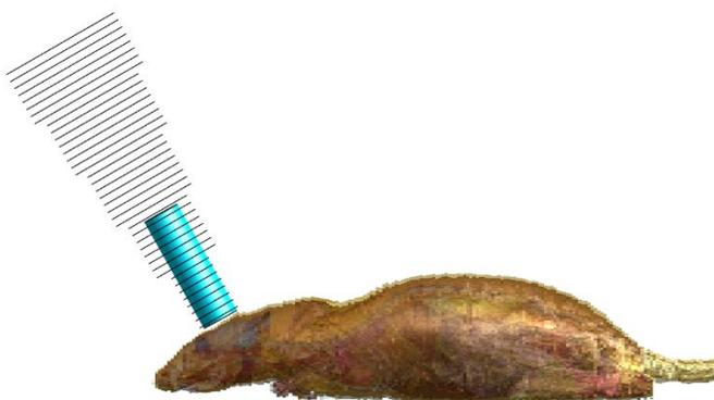
Figure 1. Focused coil along with a ferrimagnetic material, positioned on a small male rat model.
