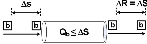
(b) Service time of the link ( $Q_b$ ) is less than or equal to the original intra-packet gap ( $\Delta S$ )
