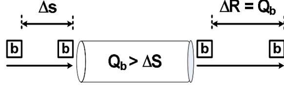
(a) Service time of the link ( $Q_b$ ) is greater than the original intra-packet gap ( $\Delta S$ )
