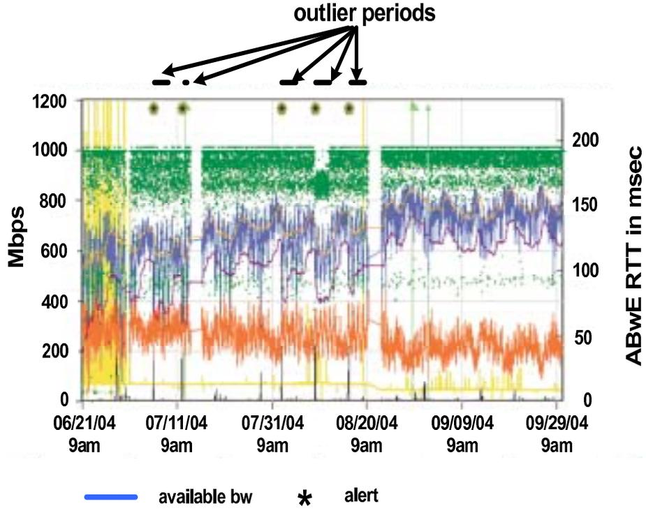
Figure 5: Detected by a modified “plateau” algorithm, periods in which available bandwidth on the path between Stanford University and the server node1.cacr.caltech.edu was significantly low.
