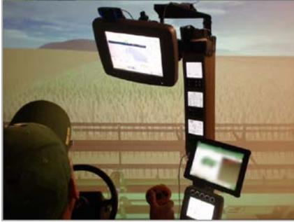
Figure 1. Harvest information displayed on four primary displays. The top display showed GPS navigation information, the three small stacked displays (corner post) showed combine diagnostic information, the iPad mounted above the arm rest displayed the Advisor/Director interface being tested, and the bottom display (the command arm) showed the current yield rate.
