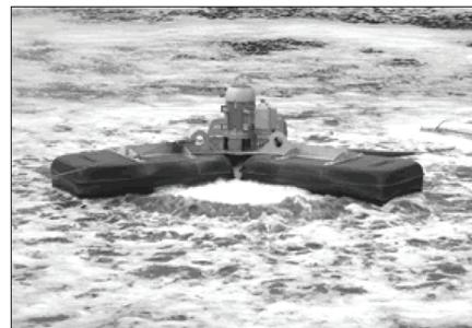
Figure 3. A down-draft aeration unit with a 5 HP, 3-phase motor that mechanically mixes and aerates the manure in lagoons or storage tanks.
