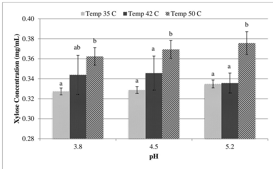
Figure 2. Xylose concentration from BluZy-P XL treatments at various pH and temperature conditions. The error bars represent the standard deviation of two replicates with three measurements each. Bars sharing same letter are not significantly different ( $p$ -value  $\leq 0.05$ ).
