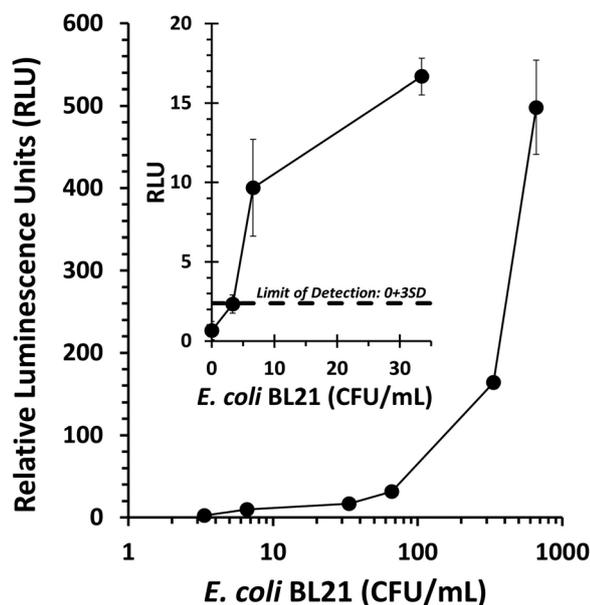
Fig. 6 Drinking water (100 mL) containing *E. coli* BL21 was used to determine the dose response of the phage-based assay. Within the range tested, increasing *E. coli* concentrations correlated with stronger bioluminescent signal. The limit of detection was defined as the negative control (0 CFU mL<sup>-1</sup>) plus three standard deviations. Data points represent the average of three replicates and error bars represent the standard deviation.
