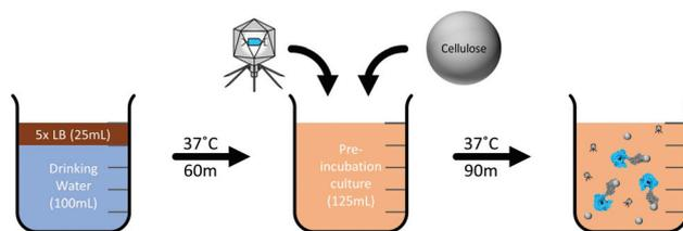
**Fig. 2** Schematic representation of detection assay. The water sample is first supplemented with concentrated growth media (5 $\times$  LB) to allow resuscitation of *E. coli*. After an incubation period, the phage and cellulose are added to the sample and the infection incubation period begins, during which expression of NanoLuc-CBM occurs. The reporter enzyme then binds to the cellulose which is collected for analysis.
