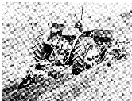
FIG. 1 Plow-plant equipment developed by C. M. Hansen and used to plant both corn and sugar beets.
