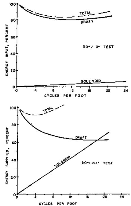
FIG. 11 and 12 Energy required by a vibrating tillage tool compared with that of a rigid tool. Tool angle, 30 deg; angles of action 10 and 20 deg, bulk density 1.23, and 17.5 percent moisture.
