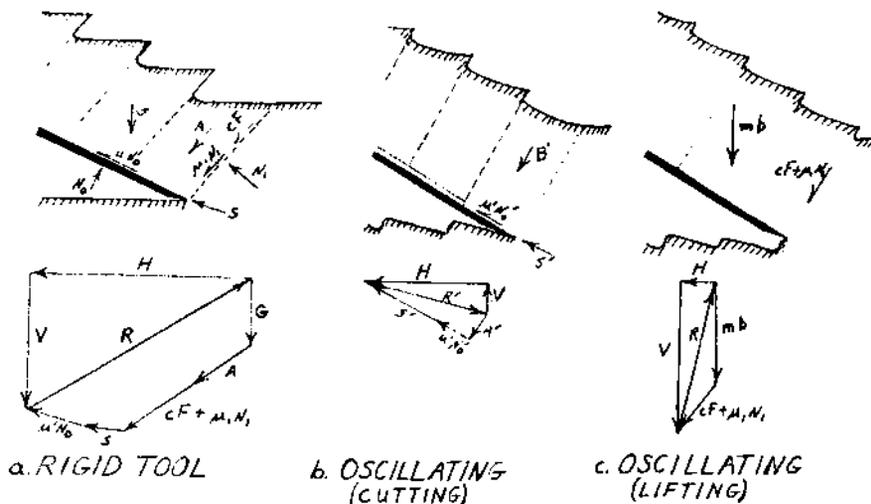
FIG. 2 Eggenmueller's representation of forces acting on a rigid tool (a) and a vibrating tool (b and c).
