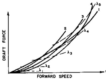
FIG. 1 Curves by Dubrovskii showing the relation between the draft of a stationary tool (curve 1) and of a tool vibrating at three frequencies (curves 2, 3, and 4) with an increase in speed  $V$ .
