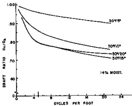
FIG. 9 Comparison of draft reduction for a tool angle of 30 deg and angles of action of 5, 10, 15, and 20 deg.
