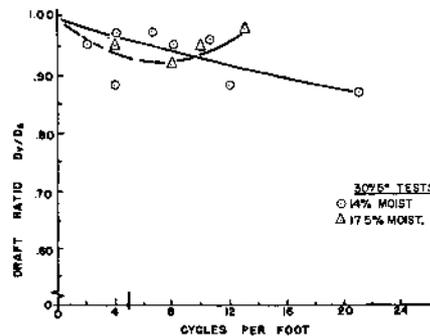
FIG. 6 Relation between the draft force of a vibrating tool ( $D_v$ ) as compared with average draft of a rigid tool ( $D_a$ ) Tool angle, 30 deg Angle of action 5 deg.
