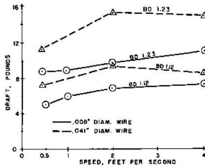
FIG. 10 Relationship between draft and velocity of 0.008-in. diameter and 0.041-in. diameter wires in soil.
