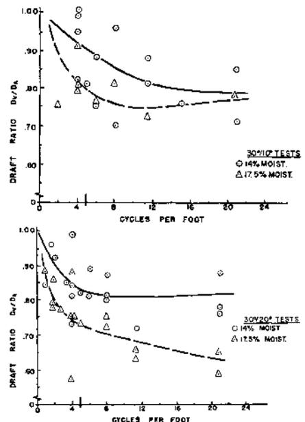
FIG. 7 and 8 Reduction in draft ( $D_v/D_a$ ) at various vibrational frequencies (cycles per foot) for a tool angle of 30 deg and angles of action of 10 and 20 deg.
