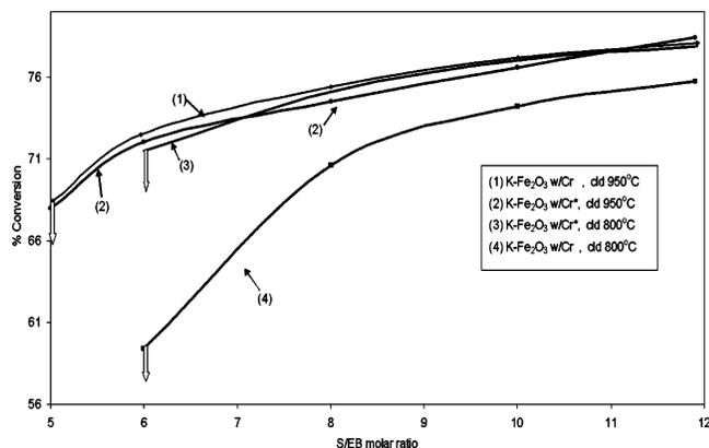
**Figure 7.** Effect of preparation calcination temperature on the isothermal performance of Cr-promoted K-Fe<sub>2</sub>O<sub>3</sub>. (The asterisk indicates Cr was added as K<sub>2</sub>CrO<sub>4</sub>.)
