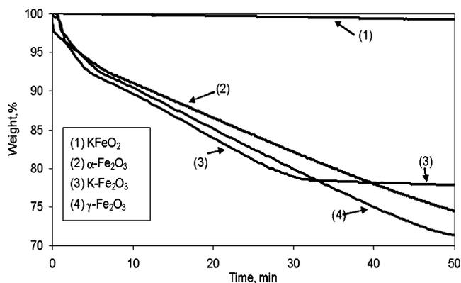
**Figure 1.** TG curves for the Fe<sub>2</sub>O<sub>3</sub> materials reduced at 630 °C and  $p_{H_2}$  = 0.057 atm.
