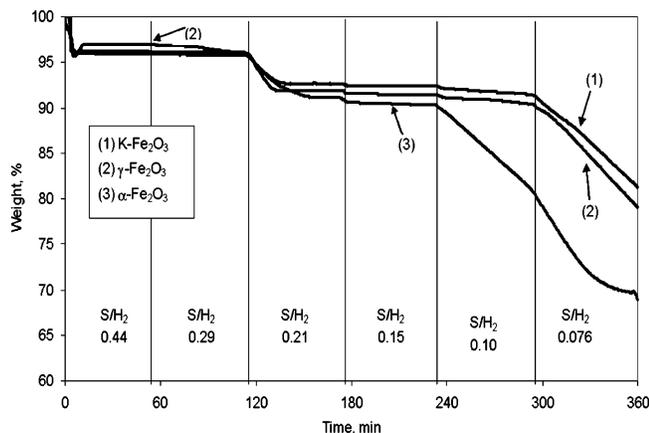
**Figure 2.** TG curves for  $\text{Fe}_2\text{O}_3$  materials at  $630\text{ }^\circ\text{C}$  and mixed  $\text{S}/\text{H}_2$  with  $p_{\text{H}_2} = 0.057\text{ atm}$ .
