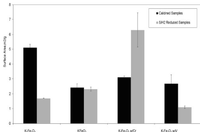
**Figure 5.** Sample surface areas after calcination at 800 °C and exposure to  $S/H_2 = 0.076$ .
