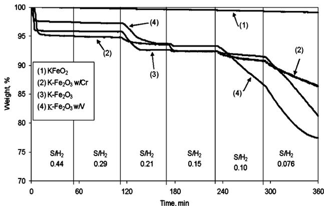
**Figure 4.** TG curves for copromoted  $Fe_2O_3$  materials at mixed steam/ $H_2$  conditions.
