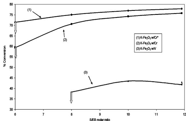
**Figure 6.** Conversion for decreasing S/EB ratios in an isothermal reactor (600 °C, 0.75 atm) with the arrows showing the point of stability loss. (The asterisk indicates Cr was added as K<sub>2</sub>CrO<sub>4</sub>.)
