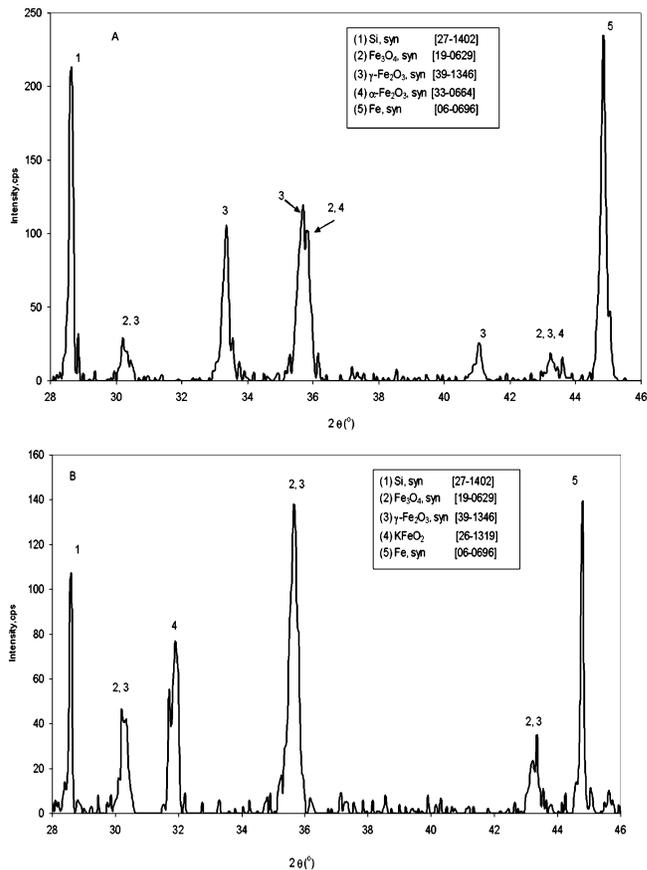
**Figure 3.** (a) XRD data for  $\alpha-Fe_2O_3$  removed after exposure to  $S/H_2 = 0.10$ . (b) XRD data for K- $Fe_2O_3$  removed after exposure to  $S/H_2 = 0.10$ .
