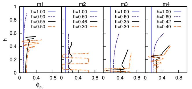
FIG. 1. The volume-fraction distribution of  $p_1$  along normalized height at selected instances during evaporation. Each color line denotes the distribution after a certain fraction of the solvent has evaporated. The modes are denoted as m1, m2, m3, and m4.
