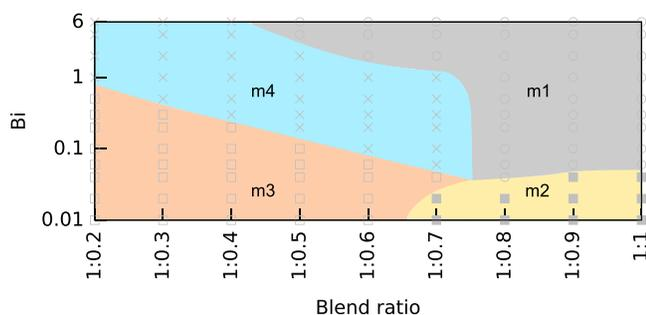
FIG. 4. Mode diagram mapping fabrication variables to four initiation modes of phase separation.
