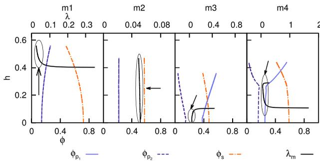
FIG. 2. Morphology evolution (1D profiles) for four modes of phase initiation (m1 to m4). Conditions just before phase initiation (1D profiles of volume fractions of three main components and the corresponding  $\lambda_m$ ). Plot corresponds to following blend ratio and Biot number: (m1) 1:1 Bi = 1.0, (m2) 1:1 Bi = 0.01, (m3) 1:0.2 Bi = 0.2, (m4) 1:0.4 Bi = 0.5.
