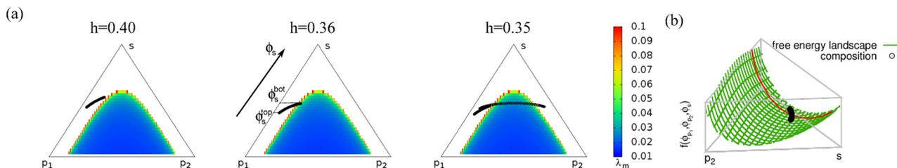
FIG. 3. (a) Morphology evolution for mode m3 of phase separation. (b) Homogenous energy landscape with distribution of composition (black dots) overlaid and iso-contour following blend ratio 1:0.2 (red curve). For temporal evolution of composition path see movie M5 in Ref. 23.
