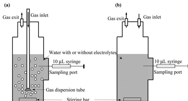
**Figure 1.** Schematic of the CO–water mass-transfer experimental apparatus: (a) for the enhancement in  $k_L a$  and (b) for the enhancement in  $k_L$ .
